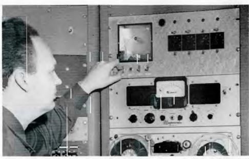
The author, Lyle Thompson, checks his cam-operated Automatic Starter Switch, used at Keating Studios to control the operation of a bank of Magnecorders which record NBC, ABC and MBS programs for Midnight Sun Beoadcasting Company.
