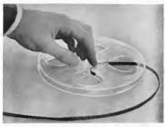
B. Drop tape into slot, leaving about 1 inch projecting beyond the hub with tape slack on both sides of recording head. Then press the "start" button. Tape will grip and hold firmly . . . no need to turn reel by hand to anchor free end.
