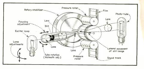
types. They consist of 5000 or 7000 cycle tones in either variable area or variable density. The variable density is more sensitive to small changes in azimuth and is to be preferred for this test. Correct azimuth and sharp focus are both manifest by maximum output as observed with a volume indicator. Some reproducers have the azimuth pre-adjusted at the factory and should not be tampered with. Usually from 100 to 200 feet of the film is all that is required.
