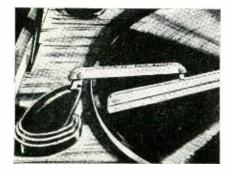
not include a pneumatic chip removal system. It relieves the operator of the responsibility of continually brushing the thread out of the way of the recording stylus, and prevents the possibility of spoiled recordings due to thread tangle.
