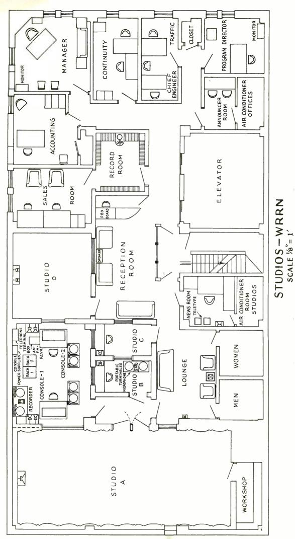
Fig. 2—Floor plan for WRRN, Warren, Ohio. This compact, efficient layout will be of interest to AM-FM broadcast station operators. A single Master Control Room services the four studios grouped around it.
