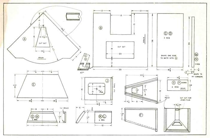
Fig. 5. Details of the pieces which comprise the lower cabinet, speaker well, and tube enclosure.
