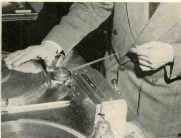
Fig. 3, left. Marked tape ready to be cut at the first mark. Use a slicing action when cutting to avoid fracturing the tape ends. Fig. 4, right. Running off tape to be discarded. This section of the tape is between points previously marked.
