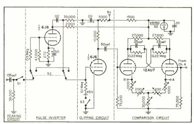
Fig. 4. Schematic of inverter, clipper, and comparison circuit.
