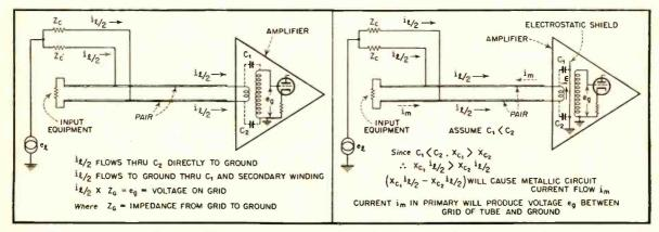
Fig. 8 (left). Conversion of longitudinal current to a metallic circuit voltage by interwinding capacitances in input transformer. Fig. 9 (right). Conversion of longitudinal current to metallic circuit voltage by capacitance unbalance.
