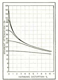
Fig. 3. Apparent attenuation vs harmonic distortion of the test signal for constant fundamental frequency attenuation levels of 60, 50, 40, 30, and 20 db.
