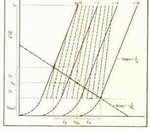
Fig. 3. Idealized plate and cathode-follower characteristics for a triode.
