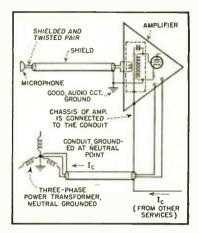
Fig. 14. Multiple grounding method.
