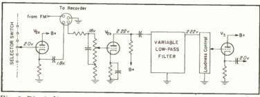
Fig. 1. Block diagram to show basic circuit before refinements of design provide complete schematic.
