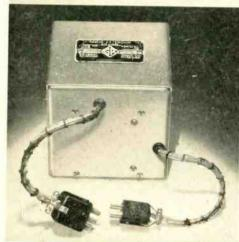
• The normal range of this oscillator is 20 to 15,000 cycles. This Range Extension Unit lowers the range by a full decade to 2 to 15 cycles, greatly extending the oscillator's usefulness to frequencies considerably below those heretofore practicable.
