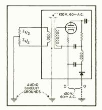
Fig. 13. Analysis of source of noise in an a.c.-d.c. amplifier.
