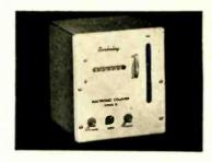
Model 10 is unique in the fact that all circuits have been developed around a single tube type, the 12AU7, to facilitate replacement. Selenium rectifiers provide d.c. power supply. Manufactured by Berkeley Scientific Corporation, 2200 Wright Ave., Richmond, Calif.
