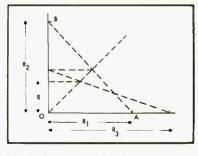
Fig. 3. Construction for three resistances in parallel.
