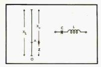
Fig. 9. Inductance and capacitance in series invalve anly vertical straight lines.
