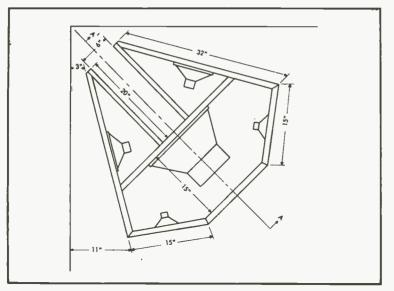
Fig. 2. Plan view of the horn-loaded cabinet, showing the two mid-range cones in the return sides, two tweeters on two front panels, and the position of the 15-in. woofers.
