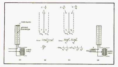
Fig. 1. The development of the distortionless push-pull electrostatic loudspeaker unit: (A) the basic arrangement with its drive unit; (B) this produces a linear driving force on the diaphragm, provided the diaphragm does not mave; (C) when the diaphragm moves, the driving force becomes non-linear; (D) preventing the charge flow, mentioned in the text, by means of the resistar R, eliminates, or reduces, this nonlinearity of driving force.
