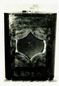
Fig. 2. With the "furniture" front panel removed, the arrangement of baffle, distributed ports, and loudspeaker protective screen can be seen clearly.
