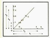
Fig. 4. Construction for four resistances in parallel.
