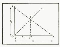
Fig. 1. Graphical solution for two resistances in parallel.
