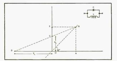
Fig. 10. Construction for capacitance and inductance in parallel.
