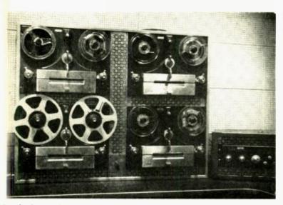
Fig. 3. Four Berlant tape-transport mechanisms and ane amplifier comprise new setup giving same advantages aver alder equipment.
