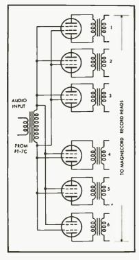
Fig. 1. Six separate output stages fed by the same input transformer eliminate the problem of interaction between bias circuits.
