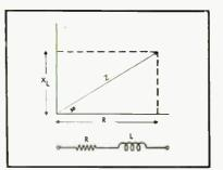
Fig. 7. Construction for resistance and inductance in series occupies different quadrant from that with capacitance.
