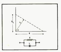
Fig. 8. Resistance and inductance in parallel network, which is handled similarly to that of Fig. 6.
