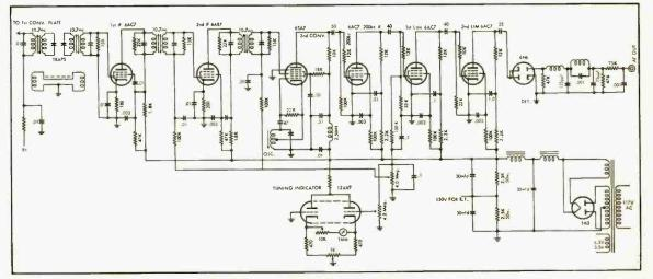
Fig. 1. The circuit schematic for the outboard i.f. amplifier. The second i.f. is at 200 kc and the detector is a frequency counter. Some old hands at audio may feel timid about tackling r.f. circuits, but there is nothing hard about it.
