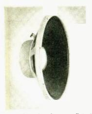
Model D130 JBL Signature Extended Range Londspeaker has cast frame, 15" diameter shallow curvilinear cone, 4" voice coil and dural dome.
