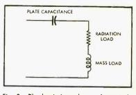
Fig. 2. The basic impedance elements in an electrostatic loudspeaker unit. This is not complete, but shows the principal elements.
