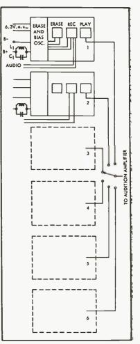
Fig. 2. Block diagram of connections to play heads of six recorders to permit audition of any one of them at will.
