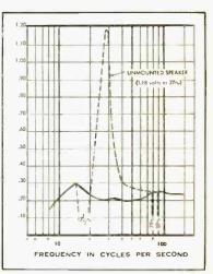
Fig. 5. Impedance curves of loudspeaker enclosed in the housing described by the author, and in open air (dotted curve).
