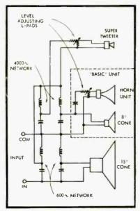
Fig. 3. Simplified schematic of the complete system. Section enclosed in dotted
