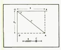
Fig. 5. Diagram representing resistance and capacitance in series.
