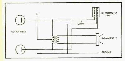
Fig. 3. Bosic method of connecting a dynamic and an electrostatic unit to the same amplifier output as a two-unit system.
