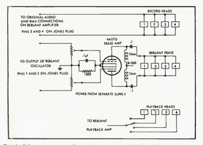
Fig. 4. Using one erase oscillator and an erase amplifier enables the statian to employ only one amplifier to record an four machines simultaneously.
