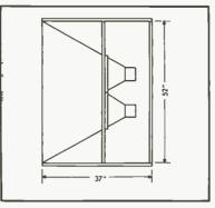
Fig. 3. Section through A-A of Fig. 3 to show flare at top and bottom of main horn.
