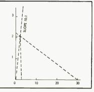
Fig. 2. When values differ widely, the scales may be changed and the transformation line is therefore no longer at an angle of 45 deg.
