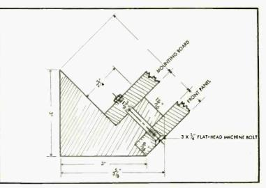
Fig. 4. Details of the front panel, speaker mounting board, and the hardwood corner post to show how the front corner of the cabinet is assembled.
