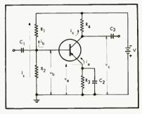
Fig. 2. By the addition of the voltage divider R1-R2, the potential of the bass is held fairly constant even though the emitter current may change appreciably.
