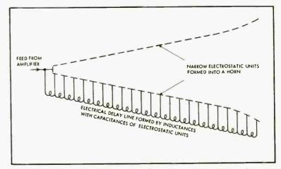
Fig. 4. The basis for a possible future development of a more efficient electrostatic horn type unit, proposed in the text.
