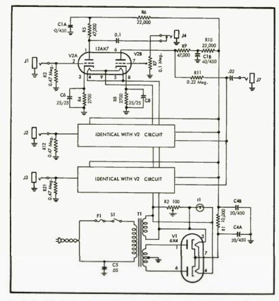
Fig. 1. Simplified schemotic of three-channel mixer-amplifier which is flexible in application.
