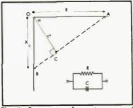
Fig. 6. Construction for resistance and capacitance in parallel.
