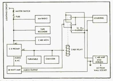
Fig. 2. Block diagram of the a.c. supply circuits and the speaker switching for the entire system.
