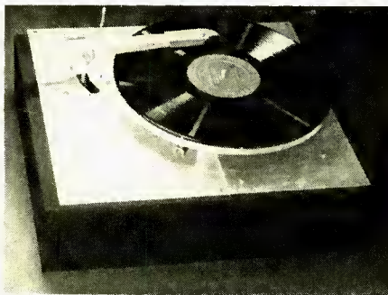
Fig. 4. Three-quarter view of device in operation. Notice slot to accommodate the movable pickup arm mount post.
