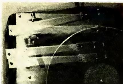
Fig. 3. Multiple exposure of device in operation showing pickup arm on the rest and in successive positions on the record. Note that the arm is tangent in all positions.
