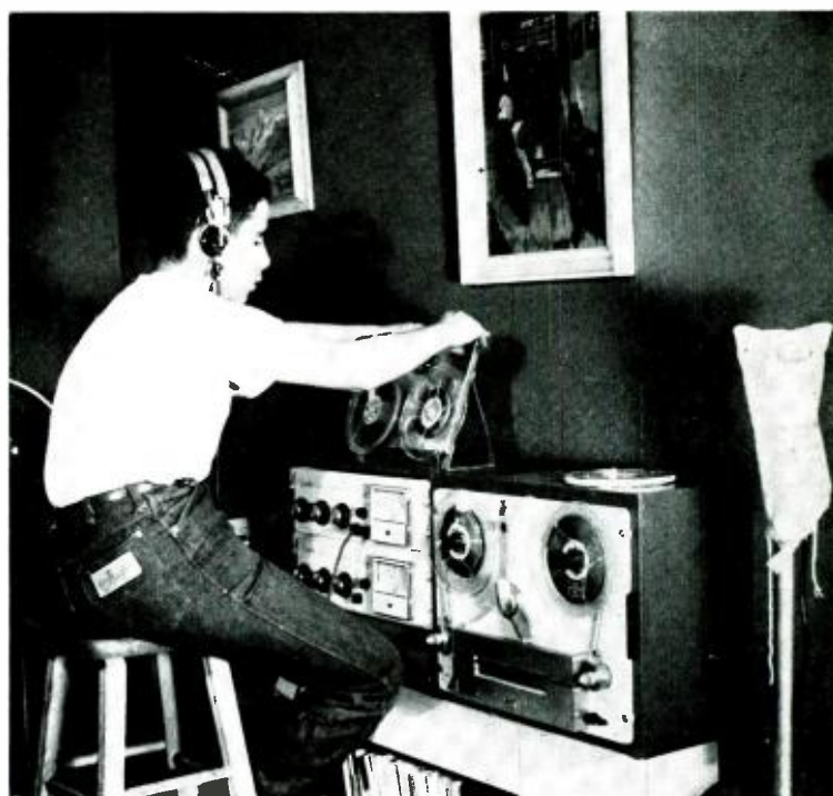
Inserting Pauses in Continuous Speech Records. Output of Viking goes to Channel 1 input of Concertone; latter runs continuously, while Viking is stopped at the end of each sentence or phrase for the desired pause.
