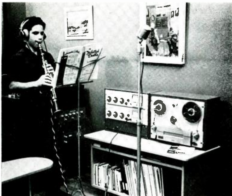
Making a Duet. Larry plays the second part of a duet along with the first part recorded previously by his instructor or by himself on Channel 1. Both parts are recorded together on Channel 2.
