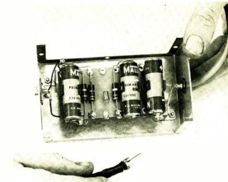
Fig. 3. Close-up of internal construction. Battery clips specified in parts list eliminate need for soldering batteries in place.
