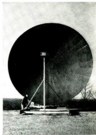
Experimental antenna used in early over-the-horizon UHF radio transmission research. Research extended transmission from 30 miles line-of-sight to 200 miles.
