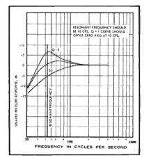
Fig. 1. Response of o direct-rodiator speaker system, in the region of resonance, at different values of Q of its mechanical system, (After Beranek)
