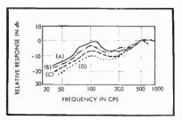
Fig. 8. Effect of restricting the solid angle seen by a loudspeaker. The top curve (A) is for a solid ongle of 45 deg.; each succeeding lower curve represents an increase of the solid ongle by a foctor of 2. (After Beranek)
