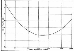
Fig. 6. Noise factor vs. source resistance for a selected 2 N 1 3 9 transistor.
