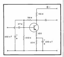
Fig. 11. Temperature-compensated transistor stage.
