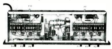
Fig. 7. Bottom view of completed amplifier chassis.
