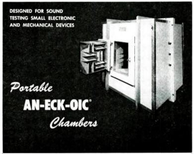
Model #545-250 as shown (outside dimensions  $65" \times 541/2" \times 65"$ , interior free field dimensions  $33" \times 22" \times 33"$ ) is designed for a low-frequency cut-off of 250 cps. Chamber is mounted on Korfund spring vibro-isolators.
