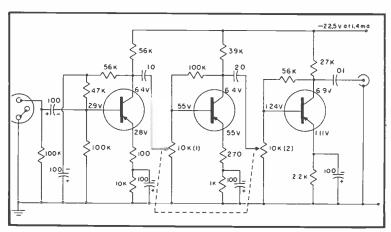
Fig. 12. Experimental microphone amplifier,
