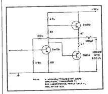
Fig. 13. Complementary-symmetry output stage.
