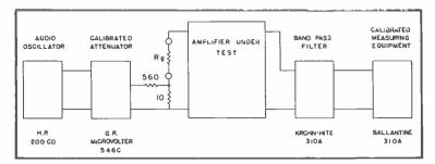
Fig. 14. Noise-figure measurement setup.
