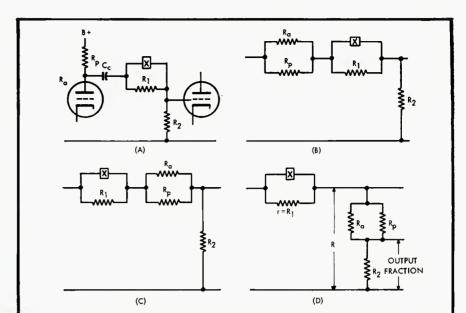
36) Fig. 15. Step by step reduction of practical circuit to basic network, for arrangements of (A) in Fig. 1, or (A) or (C) in Fig. 7.
