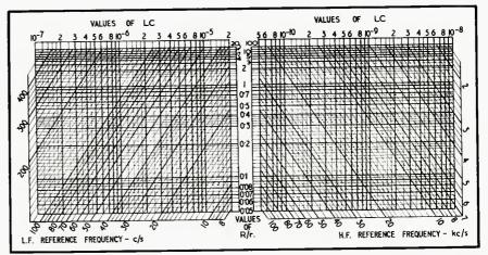
Fig. 13. Charts for giving the value of reference frequency  $f_{\phi}$ . The right hand chart applies to high-frequency peaking networks as at Fig. 10. The left part applies to low-frequency peaking networks as at Fig. 19, and the charts of Figs. 11 and 12 can also be applied for this, by taking reciprocal value of relative frequency (Fig. 12).
