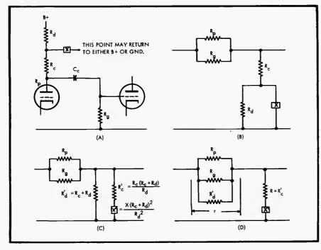
Fig. 17. An alternative practical circuit that also reduces to the same basic networks,
