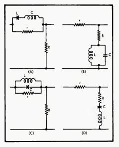
Fig. 7. Basic networks for peak and dip responses.
