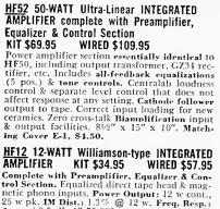
AMPLIFIER KII \$34.95 WIRED \$57.95 Complete with Preamplifier, Equalizer & Con-trol Section. Equalized direct tape head & mag-netic phono inputs. Power Output: 12 w cont., 25 w pk. IM Dist.: 1.3% @ 12 w. Freq. Resp.: 1 w: ±0.5 db 12-75,000 cps; 12 w: ±0.5 db 25-20,000 cps. 2-EL84, 3-ECC83/12AX7, 1-EZ81. 1-EZ81.
