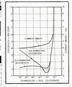
Fig. 5. Curves of distortion and current drain vs. temperature for a 0-level 400cps signal.
