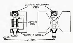
Fig. 7. Diagram of internal elements of the Grado cartridge.
