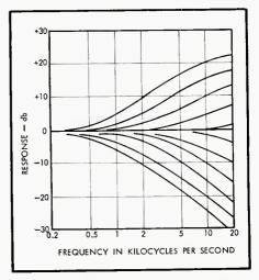
Fig. 4. Measured response of circuit of Fig. 2 for various treble-control settings.
