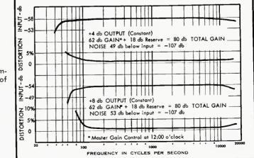
Fig. 5. Performance curves of the amplifier.
