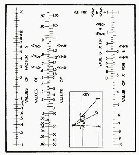
Fig. 9. Nomogram for quick computation of design point on peak and dip responses indicated in Fig. 8. The key clarifies the method of use.
