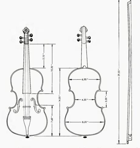
Fig. 1. With the dimensions shown here, it should be possible to work out most of the acoustic formulas to determine performance. Needed are the heights of the sides—at upper and center bouts, 1.20 inches; at lower bouts, 1.25 inches.
