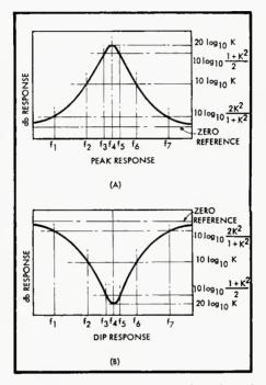
Fig. 8. Essential dimensions of peak and dip response characteristics.
