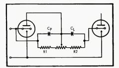
Fig. 6. Basic circuit for the bass control.
