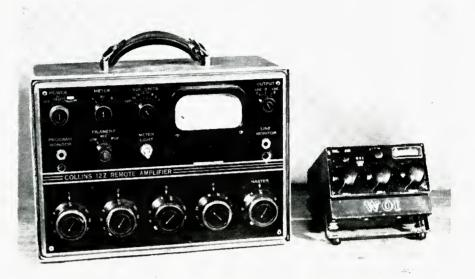
Fig. 1. The transistorized remote unit developed at WOI shown alongside a conventional tube-type Collins 12Z remote amplifier.
