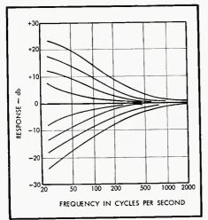
Fig. 3. Measured response of circuit of Fig. 2 for various bass-control settings.
