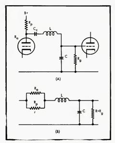
Fig. 18. Reduction of practical high-frequency peaking circuit to basic network of Fig. 10.
