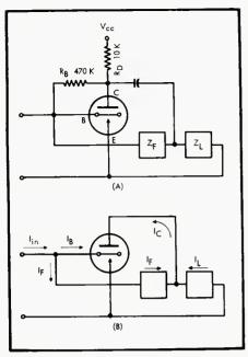
Fig. 5. Transistor feedback circuit for obtaining stabilized current gain approximately equal to Z<sub>F</sub>/Z<sub>L</sub>.
