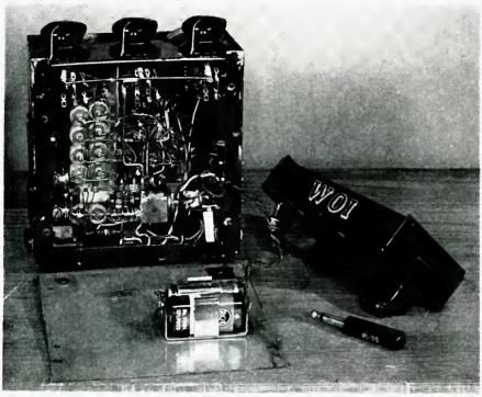
Fig. 3. Bottom view of chassis with cover. Note mounting for internal batteries. thereby raising the control knobs to a reasonable and comfortable operating height. Notches in the bottom plate serve to keep the lid in place there.
