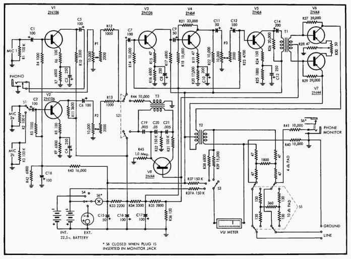
Fig. 4. Schematic of the transistorized remote amplifier.
