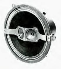
cently introduced in the United States. The dual-tweeter system affords 120 deg. dispersion. Constructional features include a heavy cast-aluminum frame, cloth cone suspension, and Fibreglass voice-coil form. Imported and distributed by United Audio Products, 202 E. 19th St., New York 3. N. Y. J-14
