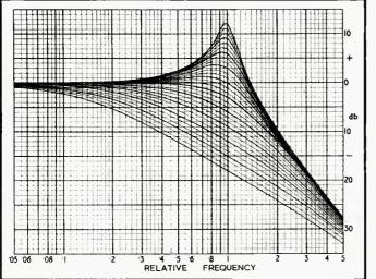
Fig. 12. The poss i b l e response curves for the network of Fig. 10. The chart of Fig. 11 identifies the required curve by the boost or attenuation at reference frequency (shown here as 1), which is  $f_{\phi}$  of equation (19). itance in the circuit.
