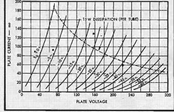
One obvious thing to be done is to get the greatest gain possible from the stage. Since the stage is excited by a signal equal to the output swing plus the grid swing, we can reduce the grid swing required by selecting power output tubes having the optimum characteristics.
