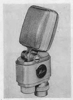
Fig. 5. The Reslo "Celeste" microphone, with on-off switch in the base,
