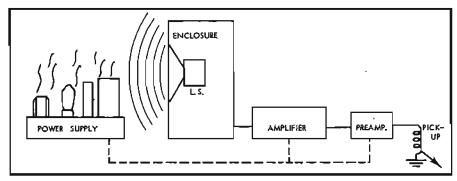
Fig. 3. Utilizing excessive voice-coil travel to provide cooling breeze for amplifier.
