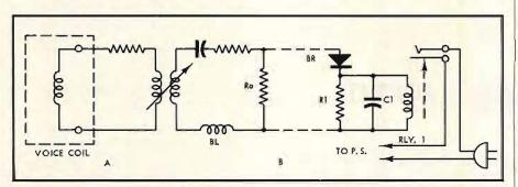
Fig. 4. Feedback-type network to actuate cut-off relay.
