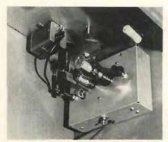
Fig. 3. Battom view of mounting board showing mechanical linkage between photo relay and base of transcription arm.
