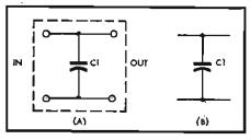
Fig. 1. Triangle-elimination network.
