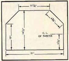
Fig. 2. Physical measurements of the Rebel IV enclasure.
