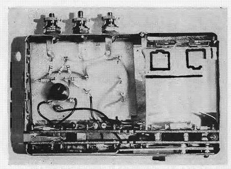
Fig. 6. Interior view of amplifier. Battery compartment is at right.
