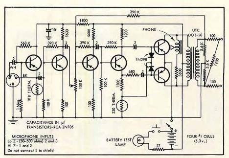
Fig. 4. Complete schematic of remote amplifier. Distortion is less than 2 per cent at + 12 dbm output, and noise is - 120 db. All transistors are RCA 2N105's.
