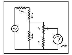
Fig. 2. Second step in measurement of damping factor involves changing of load by 10 per cent from nominal value.
