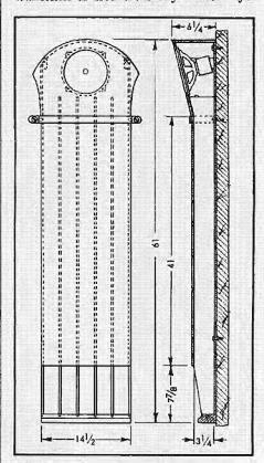
Fig. 3. Outline and sectional drawings to show dimensions of enclosure. Partitions are ¾-in. Celotex or similar softboard.
