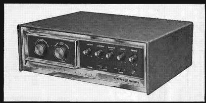
Versatile, convenient switches and controls. In this completely new and striking General Electric design you'll find every useful variation in stereo and monaural amplification, controlled swiftly and accurately. Balance control allows you to adjust for maximum stereo effect without overloading one channel when the other is cut down. New contour control boosts the bass smoothly, gradually, without increasing sound intensity. Each control handles both 20-watt channels.
