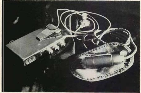
Fig. 1. Transistorized remote amplifier, manitor earphone, and microphone and case all add up to a single pocketful.
