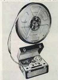
manner and is "played through." The cleaning formula with which the fabric tape is impregnated dissolves and removes iron-oxide accumulation, also picks up dust and other foreign materials from the head. The tape can be used over and over. Manufactured by Walsco Electronics Manufacturing Company, 100 W. Green St., Rockford, Ill.
