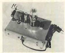
Fig. 4. Construction of shutter mechanism is illustrated by external view of photo-relay chassis.
