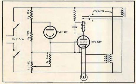
Fig. 1. Complete schematic of photo-relay circuit.
