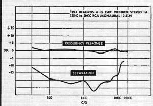
Smooth response on both stereo and monaural records, Consistently high separation between stereo channels.
