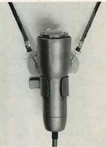
quency response." Specifications of this broadcast microphone are stated as: Frequency response, 60 to 20,000 cps; Output level, -90 db for 50 ohms impedance. -84 db for 200 ohms impedance. The unit is cased in aluminum with neutral gray non-reflecting enamel finish. For more information and complete technical specifications, write direct to The Turner Company, 909 17th St., N.E., Cedar Rapids, Iowa. A-7
