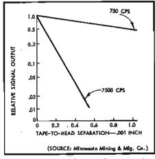
Fig. 8. Separation losses when reproducing frequencies of 7500 and 750 cps at 7.5 lps.
