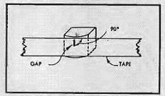
Fig. 4. Meaning of azimuth alignment.
