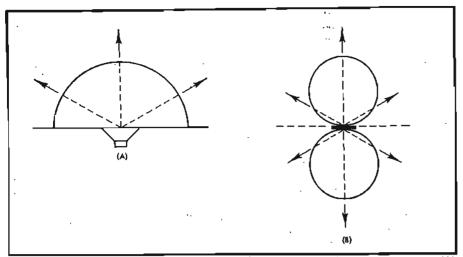
Fig. 3. Whereas baffled pistons produce hemispherical low-frequency patterns (A), baffled dipole systems (B) produce directional fields improving low-frequency prientation.
