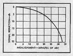
Fig. 5. Effect of azimuth misalignment upon response at 7500 and 750 cps at 7.5 ips.
