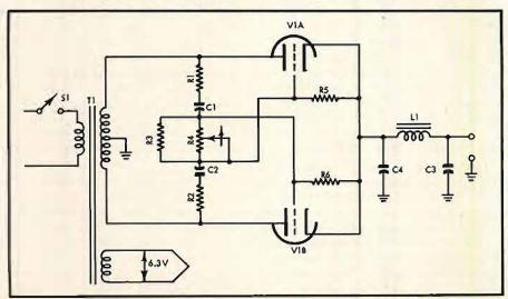
Fig. 1. Complete schematic of the variable power supply.
