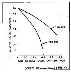
Fig. 7. Separation losses when recording frequencies of 7500 and 750 cps at 7.5 lps.
