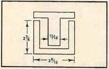
Fig. 8. Typical lamination shape.
