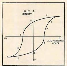
Fig. 16. Typical B/H relation for iron laminations.
