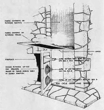
speaker section comprising 300 cubic feet. The "grille cloth" extends from floor to ceiling and is pale gray Belgian linen, the same as the draperies in the room. The size of the speaker grilles completely eliminates the feeling that there are two loudspeakers—one of the deterrents to good stereo listening, for if you can see two speakers, you can hear two, and they do not blend into a wall of sound as a good stereo system should. No trace of this sensation is felt when listening to this system.
