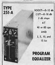
The 251-A Equalizer is a passive LCR bridged-T network with two sliding levers for attenuation and equalization, one for low frequencies and one for high. This type of equalizer has long been the standard for corrective equalization in sound recording.
