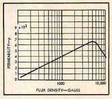
Fig. 9. Typical relation between core flux density and permeability for transformer steel.
