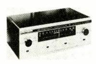
Specifications: 12 tubes; cascode front end; horiz, bar tuning indicator; controls—tuning; switches—power, a.f.c. defeat, muting, mpx noise filter, stereo-mono; freq. resp. ± 1 db from 20 to 20,000 cps; sensitivity 1.2 µv for 20-db quieting with 300-ohm antenna; stereo separation 30 db; time division stereo circuit; dimensions: 15" wide, 5½" high, 11½" dep; weight, 12¼ bbs. Price \$359.00. Altec-Lansing. .....\$256.00
