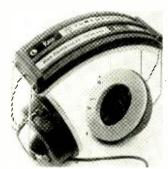
Specifications: dynamic; freq. resp. 10 to 15,000 cps; impedance 4 ohms; sensitivity 1 volt at 400 cps; will develop 127 db of sound pressure referred to 0.0002 dynes/cm²; maximum power handling 10 watts; 3 conductor plug; cold 8 ft; net weight 12 ozs. Price \$24.95. Accessories: T-5 remote control listening station. Price \$8.95. Koss Elect.
