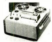
Specifications: Speeds—7½, 3¾, 1½ ips; heads—2¼-track; records 4-track stereo, 4-track mono; plays 2&4-track stereo, 2&4-track mono; reel size 7 in.; 1 motor; freq. resp.—7½ ips, ½ db from 40 to 12,000 cps; signal-to-noise ratio, 50 db; wow and flutter, 0.2% at 7½ ips. 0.25% at 3¾ ips. Inputs—2 microphone; amplifier outputs—2; speaker outputs 2, impedance 8 ohms; output power 10 watts. bimensions, 13¾ wide, 9¾ bigh, 14″ deep; weight, 34½ lbs. Price, \$319.95. Concord Elect.
