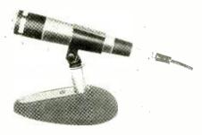
Specifications: dynamic; cardioid dir. pattern; baked enamel finish; output impedance 30/50, 150/250, 20k ohms; freq. resp. 45 to 15,000 cps; length of cable furnished 15 ft.; dimensions—1½" dia., 7½" long; weight 11 oz. Slip-on adapter mounting. Price, \$72.00. Altec-Lansing.
