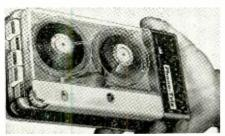
Specifications: Speeds—17% ips; heads—2½-track, records 2-track mono; plays 2-track mono; reel size 2½ in.; 1 motor; freq. resp. 1½ ips, ±3 db from 100 to 6000 cps; rewind time, 600-ft reel, 30.1 secs. Inputs—microphone, impedance 200 ohms; amplifier outputs—1; speaker outputs 1, impedance 1k ohms; output power 10 mw. Dimensions, 17½ wide, 4½" high, 7½" deep; weight, 2¾ lbs. Price. \$99.95, Matthew Stuart.
