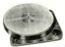
Specifications: Speeds—16%, 33½, 45, 78 rpm; rim drive; 4-pole induction motor; turntable diameter, 12"; turntable weight, 3 lbs; turntable material, aluminum; mat, rubber; wow, 0.2%; flutter 0.2%; dimensions of chassis, 12½"×10½"; clearance required above mounting board, 1½"; below, 4"; controls, speed, power; provision for arm mounting, none; over-all weight, 14 lbs. Price, \$37.50. Lafayette Radio.
