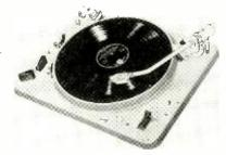
\*\*Specifications: Speeds—16%, 45, 33½, 78 rpm; rim drive; synchronous motor; turntable diameter, 13"; turntable weight, 8 lbs.; shaft diameter, ½"; turntable material, cast iron; felt mat; wow and flutter 0.3% peak-to-peak or 0.1% rms; dimensions of chassis, 15½"×19½"; clearance required above mounting board, 2"; below 7"; controls on/off, stereo selector; over-all weight, 22 lbs. Price, \$595.00. Accessories, electronic brake \$89.50. Gotham Audio.
