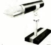
Specifications: dynamic; uni-directional pattern; output impedance 600/50k ohms; freq. resp.  $\pm$  1.5 db from 100 to 14.000 cps; sensitivity, -75  $\pm$  3 db (600 ohm); dimensions— $1\frac{1}{4}$ "  $\times$  6 7/16". Primo Co.
