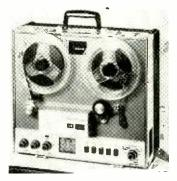
signal-to-noise ratio, 50 db; wow and flutter, 0.2% at 7½ ips, 0.25% at 3¾ ips; rewind time, 1200-ft. reel. 40 secs. Inputs—2 nicrophone, high impedance, sensitivity 1 mv; 2 high level, high impedance, sensitivity 0.1 volts; amplifier outputs—2, cathode follower phone output. Dimensions, 16¼" wide, 7¾" high, 14" deep; weight 44 lbs. American Concertone.
