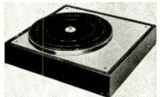
Specifications: Speeds—33½ rpm; rim drive; hysteresis-synchronous motor; turntable diameter, 12"; turntable weight, 12 oz.; turntable material, aluminum; Ring support mat; wow and flutter 0.1%; dimensions including base, 16½×15×3; provision for arm mounting, 2½" internal clearance. Price, \$59.95. Weathers Ind.
