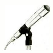
Specifications: dynamic; cardioid pattern; Acoustalloy® diaphragm material; die cast case; chrone finish; output impedance hi or 150-ohm; freq. resp. ±5 db from 50 to 15.000 cps; sensiti√ity; −57 db (1 v/dyne/cm²); cable connection 91-MC4M Amphenol or equivalent; length of cable furnished 18 ft.; dimensions −7%"×1½" dia.; weight 12 ozs.; slip mounting. Price, \$100.00. Accessories: Model 420 desk stand \$20.00; Model 355 Windscreen; \$11.00: Electro-Voice.
