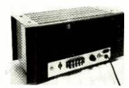
Specifications: Freq. resp. 20 to 30,000 cps ±1 db at 0.5 watts output; IHF music power output, 100 watts per channel; power output, rns, 70 watts per channel; harmonic distortion, 1% at 70 watts from ±0 to 20,000 cps; IM distortion, 1% at 70 watts; hum and noise, 75 db below 70-watt output; sensitivity, input for rated output, 0.9 volts; output impedances, 4, 8, 16 ohms; level control; 1 convenience outlet; weight, 26½ lbs; dimensions, 14¾" wide, 7¼" high, 3¼" deep. Pioneer Electric Corp.
