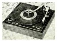
Specifications: Speeds—16%, 33%, 45, 78 rpm; rim drive; 4-pole motor; turntable diameter, 11°; rubber mat; dimensions of chassis, 13%" × 12"; clearance required above mounting board, 4%"", below, 3"; type of mounting, leveling shock nuts, controls, speed, function, tracking weight; type of pickup head, plug in; material, plastic; number of leads to head, 4; number of leads to chassis, 2 cables, Price, \$49.95, Allied Radio.
