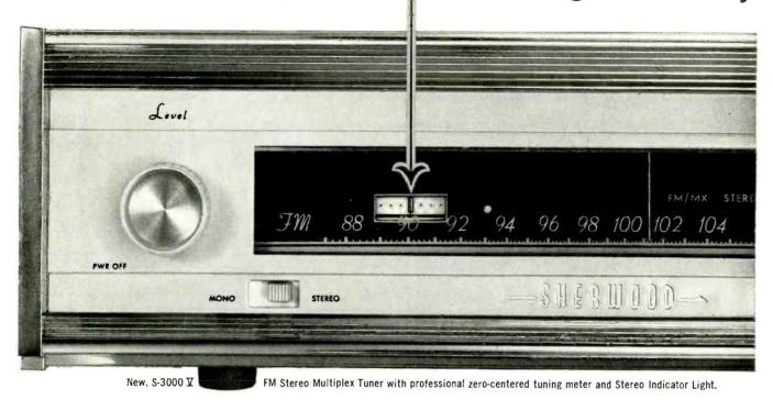
The wider band requirements for the stereo information now being multiplexed on FM channels has made precision tuning a factor more-important-than-ever in FM reception.
