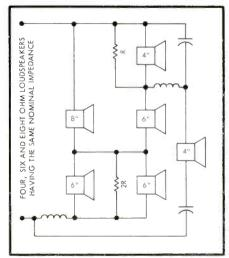
Fig. 1. As an elaboration one could take four 6-inch models for the 8-inch one, an 8-inch one for each of the 6-inch models, and four 4-inch models, thus arriving at a total of twelve loudspeakers. Note: **R** is a wire-wound resistor whose value is the same as the nominal impedance.
