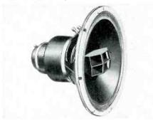
Specifications: Type, duplex; power handling capacity, 35 watts; impedance 16 ohms; frequency response, from 20 to 22k cps; magnet weight, 1.f. 40 oz., h.f., 8 oz.; voice-coil diameter, 1.f. 3", h.f. 1\%"; free air resonance frequency 25 cps. Dimensions: 15 5/16" dia.. 10" deep; weight, 37 lbs. with network. Price \$168.00. A15-2.
