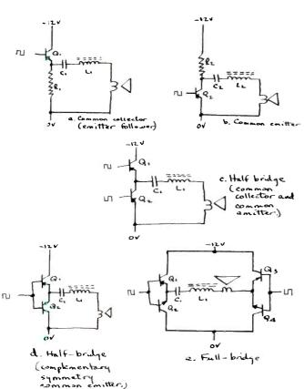
Fig. 20. Possible output stage circuits.
