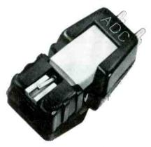
recommended tracking force—professional arms, 0.75–1.5 gms: compliance-lateral, 30 × 10–6 cm/dyne, vertical, 30 × 10–6 cm/dyne; inductance, 500 mh; d.e. resistance, 700 ohms; 4 terminals; mounting dimensions, 7/16" or ½". Price, diamond, \$60.00; replacement styli, elliptical—\$25.00; regular—\$15.00.
