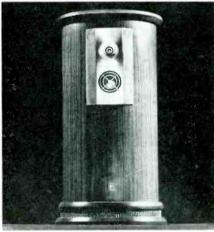
response ± 3 db from 20 to 20k cps; sensitivity (watts input for +85-db level 10 feet on axis) 1.0 watts at 1 kc; magnet weights; f. 9 lb; m.f., 2½ lb; h.f., 1 lb.; voice-coil diameters: l.f., 4"; m.f., 2¾", h.f., 1"; die cast wide angle acoustic lens for mid and high frequency direct radiators. Dimensions: 29" H, 22" diameter; weight 85 lbs.; handrubbed satin walnut \$250.00, A16-5.
