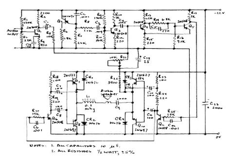
Fig. 21. Schmidt-trigger modulator amplifier schematic.
