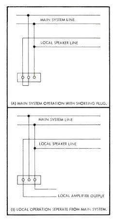
Fig. 5-2. Method of providing local tap-in for speaker system, so installed speakers can be connected, either to the main system, or for local use.
