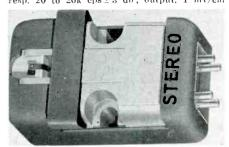
rec. velocity; channel separation, 28 db at 1 kc; recommended load, 12–47k ohms; recommended tracking force—professional arms, 1.5-5 gms; changers 2–5 gms; compliance—lateral  $4\times10$ -6 cm/dyne, vertical,  $3\times10$ -6 cm/dyne; inductance, 250 mh, d.c. resistance 800 ohms/channel; no. of terminals, 4; mounting dimensions, std.: weight 14 gms. Price, diamond, \$34.50; replacement styli, \$17.25. A11-4.
