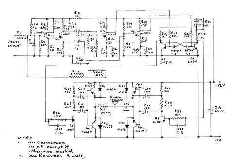
Fig. 25. Astable multivibrator amplifier schematic.
