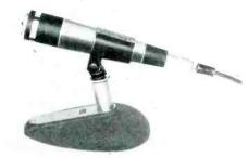
Specifications: dynamic; cardioid dir. pattern; baked enamel finish; output impedance 30/50, 150/250, 20k ohms; freq. resp. 45 to 15,000 cps; length of cable furnished 15 ft; dimensions—1½" dia., 7½" long; weight 11 oz. Slip-on adapter mounting. Price, \$72.00.
