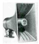
ohms; frequency response, 250 to 14k cps; EIA sensitivity 59 db; magnet weight 11.3 oz; voice-coil diameter 1.5 in.; dimensions  $11''h \times 6\frac{1}{2}''w \times 8\frac{1}{2}''d$ ; mounting, universal swivel bracket; weight, 5 lb. 9 oz. Price \$20.70. Accessories: TR3-2 25-volt line transformer, \$9.00; TR3-7 70.7-volt line transformer, \$9.00. CS4-2.
