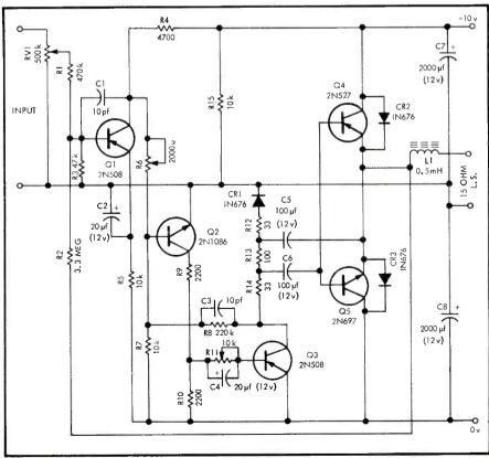
Fig. 23. K. C. Johnson amplifier schematic.
