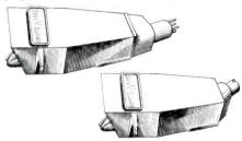
Specifications: Freq. response 20 to 17k cps ±2 db; output 2 mv; channel separation, 35 db at 1 kc; recommended load, 47k-100k ohms; recommended tracking force—professional arms, 1-3 gms, changers, 3 gms; inductance, 245mh; d.c. resistance, 410 ohms; capacitance, 250 pf; 4 terminals; mounting std.; weight, 14 gms. Price, diamond, \$52.50; replacement styli, \$17.00, A11-14.
