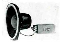
Specifications: dual concentric; power handling capacity 20 watts; impedance 16 ohms: frequency response, ±3 db from 27 to 20k cps; magnet assembly 64 lbs; L.F. voicecoil diameter 2½" (HF, 2"); free air resonance frequency 27 cps; recommended enclosure volume 1½ cu. ft. minimum. Dimensions 115%" dia. 6½" deep; mounting dimensions, (4) ¼-in. holes on 11" circle; cutout diameter 9"; weight, 9 lbs. Price \$112.75. Other features: Crossover weight 2½ lbs.; finish, hard enamel. A15-17.
