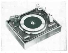
ribbed with chrome insert mat; dimensions of chassis. 16¾ "×14½"; clearance required above mounting board. 6"; below, 2½"; type of mounting, barrel springs; controls. manual and auto on/off; automatic cycling time, 10 secs at 33½ rpm, 3½ secs at 78 rps; type of pickup head, plug-in 4 pin; material, plastic;
