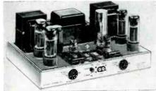
Specifications: Freq. resp. 10 to 40k cps; ± 0.5 db at 1 watt output; power output, rms, 35 watts per channel; harmonic distortion, 1% at 35 watts, +1 db from 20 to 20k cps; M distortion, 1% at 35 watts; hum and noise, 90 db below 35-watt output; sensitivity, input for rated output. 1.3 volts: damping factor. 15; output impedances, 4, 8, 16 ohms; controls, dual bias adjust;
