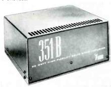
Specifications: Freq. resp. 20 to 20k ±1 db; IHF music power output, 50 watts; harmonic distortion, 1.5% at 40 watts from 25 to 10k eps; hum and noise, 90 db below 50-watt output; sensitivity, input for rated output, 0.45 volts; damping factor, 7.5: output impedances, 4, 8, 16, 125 ohms, 70v; controls, level; switches, protective circuit; weight, 15 lbs; dimensions, 9¾" wide, 5" high, 9¾" deep; price, \$252.00. A1-2.
