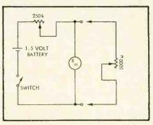
Fig. 3. The meter resistance  $R_m$  is equal to the resistance of the 5k pot when the meter deflection is reduced to one half full scale.
