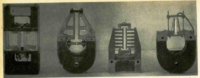
Fig. 2. Skeletons of various ribbon microphones. Left to right: RCA 44BX; RCA 44A; the author's first design; the author's "calibration" model.
