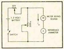
Fig. 2. Full-scale meter current  $l_m$  is measured directly with another ammeter. The reference meter must be reasonably accurate.
