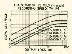
Note how losses pile up as skew angle increases. And as you would guess, the losses are in proportion to the frequency. Higher frequencies, higher losses. Same principle, really, as an azimuth loss.
