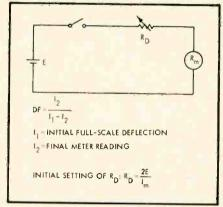
Fig. 10. The damping factor of a meter is the ratio of the final reading to the amount of overshoot.
