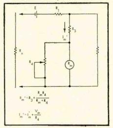
Fig. 8. An improved ohmeter circuit which compensates for aging batteries with a minimum effect upon  $R_h$ . Use  $R_m'$  and  $I_m'$  in place of  $R_m$  and  $I_m$  in the equations of Fig. 7.
