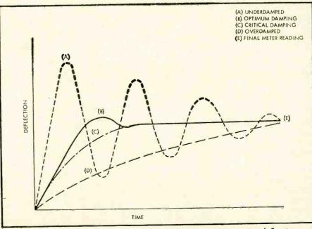
Fig. 9. The effects of various amounts of damping upon meter deflection.
