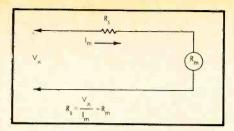
Fig. 4. The voltmeter indicates voltage by measuring the current through a series resistor,  $R_s$ .
