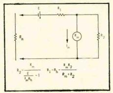
Fig. 7. The ohmmeter indicates resistance by measuring the current through the unknown resistor,  $R_x$ .
