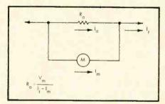
Fig. 5. The ammeter is a current divider which passes  $I_m$  through the meter and shunts all the rest of the total current,  $I_t$ , through resistor  $R_t$ .
