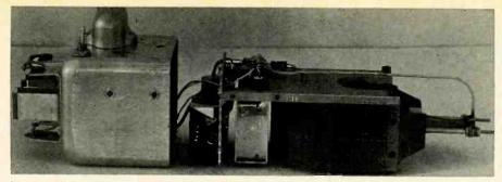
Fig. 4. Self-contained output system, showing the emitter-follower, and behind it, the transformer. The amplifier adjoins the magnet.
