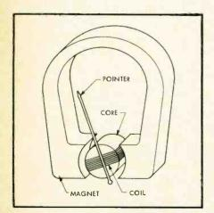
Fig. 1. The meter core is almost completely surrounded by the uniform field of a permanent magnet. The deflection of the pointer is proportional to the current in the coil.
