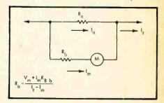
Fig. 6. Modified ammeter allows larger value of R<sub>a</sub> by increasing total voltage drop across instrument for full scale deflection.
