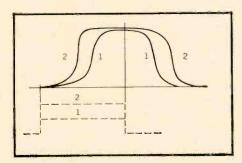
Fig. 2-4. Increasing base-drive current usually shortens delay time but lengthens storage time (curves 2 as compared with curves 1).
