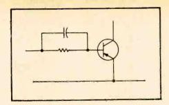
Fig. 2-3. A bypass capacitor can sometimes shorten either delay or storage time, or both.
