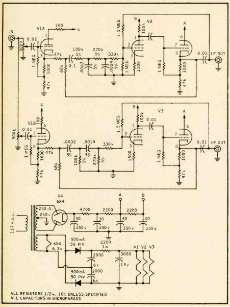
Fig. 8. Schematic of 350-Hz electronic crossover.
