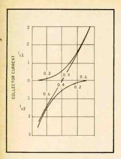
Fig. 4. Push-pull stage improves linearity by complementary matching of curves.
