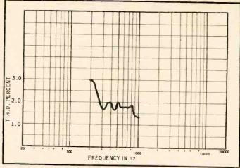
Fig. 4 (left). Averaged frequency response of bass-horn measured at a number of points in the listening room. Fig. 5, (right). Curve of harmonic distortion with 10-watt input.
