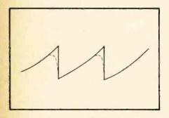
Fig. 2-11. Effect of using coupling diodes, in multivibrator output, with inadequate forward conduction (too high forward resistance): solid line, required pulse shape; dashed line, result of high forward resistance in diodes.
