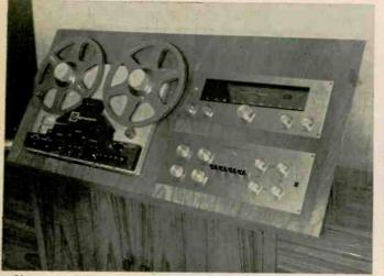
Close up of the control panel which accommodates the tape recorder, tuner, and preamp.
