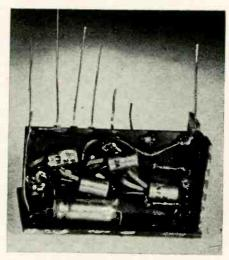
Fig. 8. View of the right side of the amplifier after further steps, including mounting of the transistors.
