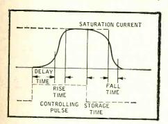
Fig. 2-1. A sample of the kind of output pulse generated by one type of transistor, to illustrate the meaning of the four time constants associated with transistors operating in switching mode.
