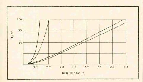
Fig. 8. By juggling source resistor values as well as emitter resistor, performance can be improved as in this set of curves.
