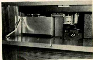
Electronic drive compartment under right turntable, with the drive unit shown at the left and the Papst turntable motor at the right.
