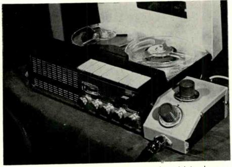
Fig. 1. Converted Uher 4000 Report-S, with output coupling unit/microphone preamp at the right.
