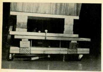
Close-up view of the ratchet roller-lift showing its application. The cabinet is raised sufficiently to permit placing wood blocks on the lift, holding it clear of the floor with complete safety for moving.
