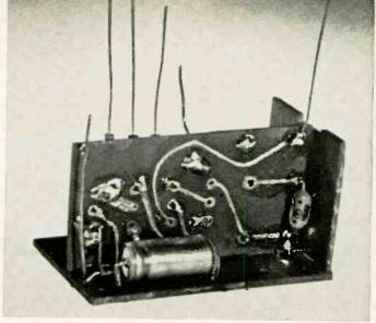
Fig. 6 (left). Initial step in construction with  $L_1$  and several of the resistors in place. Note end board, flush against  $L_1$  and the center board (1). Fig. 7 (right) earlier steps in construction as seen from the opposite side.
