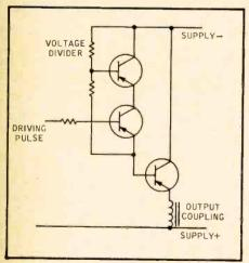
Fig. 2-8. Using two lower-voltage-rated transistors to serve on higher voltage by series connection. The two drive transistors shown here can withstand the full supply voltage needed to drive the output as an emitter follower, although their individual voltage rating is not high enough.
