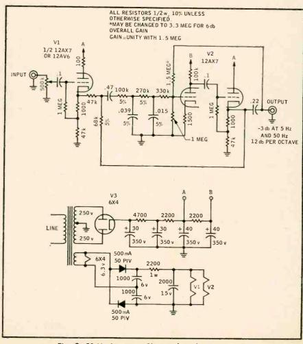
Fig. 9. 50-Hz low-pass filter in bass-horn circuit.
