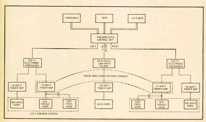
Fig. 7. Block diagram of complete audio system.
