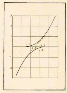
Fig. 5. Quiescent current (and dissipation) are reduced by lowering bias on stage of Fig. 4.
