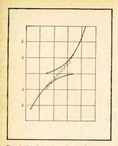
Fig. 6. Similar curve obtained with two actual transistors, in contrast to previous curves plotted from specifications for a "typical" transistor.
