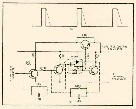
Fig. 2-12. Some details in development of satisfactory pulses: a. sloping trailing edge that occurs with no positive feedback to sharpen switching (dashed line); solid line shows effect of positive feedback; b. alternative ways of connecting positive feedback (values are those successfully used in those locations); in dashed ellipse is modified coupling between mixer and drive stage, to sharpen trailing edge of drive-stage pulse.
