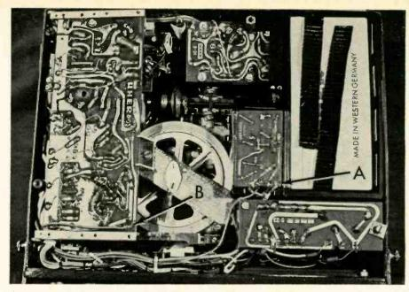
Fig. 14. Underside of Uher 4000 Report-S with new amplifier in place. Point indicated by "A" is where head connection is made. "B" shows where —6 volts is obtained from printed circuit of the recorder.
