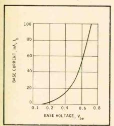
Fig. 1. Typical power-transistor characteristic in which slope becomes essentially constant at maximum signal.
