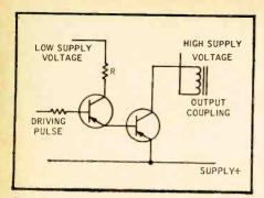
Fig. 2-7. Use of different supply voltages, when the output stage is collector coupled (grounded emitter). Resistor R limits drive-stage collector current, which is essentially output-stage base current.
