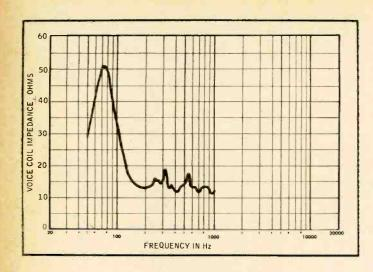
Fig. 6. Voice-coil impedance of bass-horn driver.
