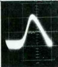
Fig. 8—Evidence of too narrow a bandwidth ('scope settings are the same as in Fig. 7).
