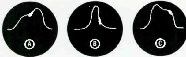
Fig. 7—Typical i.f. response, measured at the AGC take-off point of a receiver.
