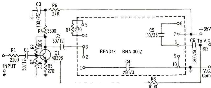
Fig. 4. Schematic of the completed unit with an additional stage to provide for more feedback to increase output into an 8-ohm load. The integrated-circuit amplifier is shown inside the dotted lines.
