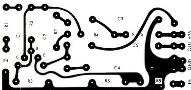
Fig. 5. Layout for the printed circuit board shown full size. This drawing may be copied exact size to make your own printed circuit board.
