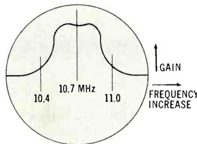
Fig. 5—By introducing unmodulated 10.7 MHz from a second generator (loosely coupled), a "pip" appears on the response curve. This aids in "centering" the response at 10.7 MHz.
