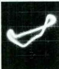
Fig. 10—"Classical" S-curve display measured at detector output. The linear portion of the curve in this case extends  $\pm 120$  kHz above and below center "zero" point.
