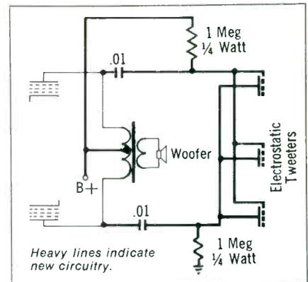
Fig. 1—Connections for driving electrostatic tweeters from vacuum-tube amplifiers.
