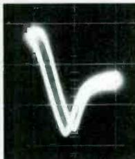
Fig. 12—Another example of improperly aligned ratio-detector secondary.
