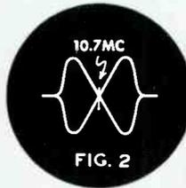
FM IF ALIGNMENT USING FM SIGNAL GENERATOR AND OSCILLOSCOPE—SELECTOR IN FM POSITION
