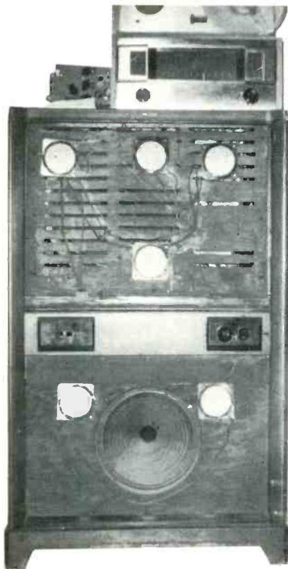
Fig. 3—Author's loudspeaker system with grille cloth removed to show electrostatic speakers. At bottom is rear of the enclosure. The upper unit is a transistor amplifier; the lower unit is the power supply for electrostatic speakers.
