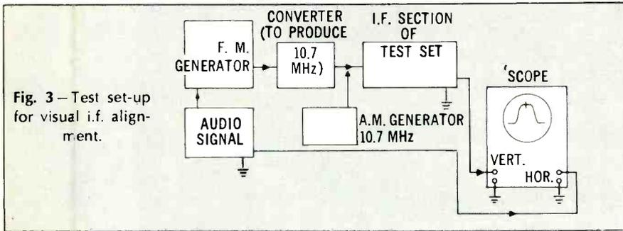
Fig. 3—Test set-up for visual i.f. alignment.
