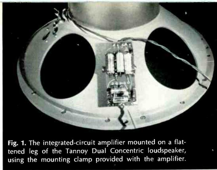
**Fig. 1.** The integrated-circuit amplifier mounted on a flattened leg of the Tannoy Dual Concentric loudspeaker, using the mounting clamp provided with the amplifier.
