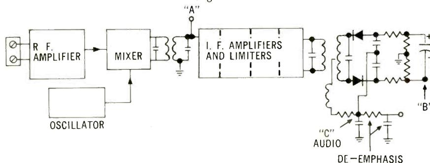
Fig. 2—Equivalent test points to those shown in Fig. 1 for typical discriminator circuit.
