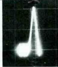
Fig. 9—Assymetrical i.f. response due to improper stagger tuning.
