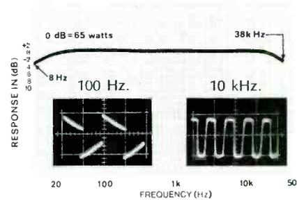
per channel, as shown in Fig. 6. Tone control range was adequate and quite symmetrical (See Fig. 7). The low and high-frequency filters are also plotted in Fig. 7 and are of the 12 dB/octave type, making them useful and meaningful.
