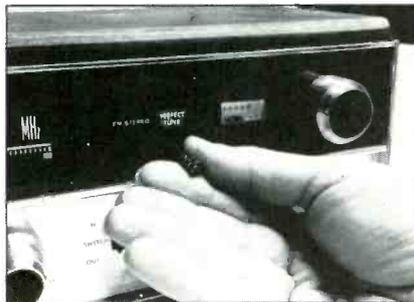
The Model 342C's control features are: dual bass and treble, stereo balance, tape monitor, speakers #1 on/off, speakers #2 on/off, power on/off, volume control, volume compensation, muting, noise filter, and mode switch, as well as a signal strength meter, stereo indicator light, and front-panel stereo headphone output, plus the aforementioned automatic tuning indicator.
