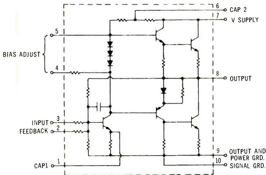
Fig. 3. Internal circuit of the integrated-circuit power amplifier.
