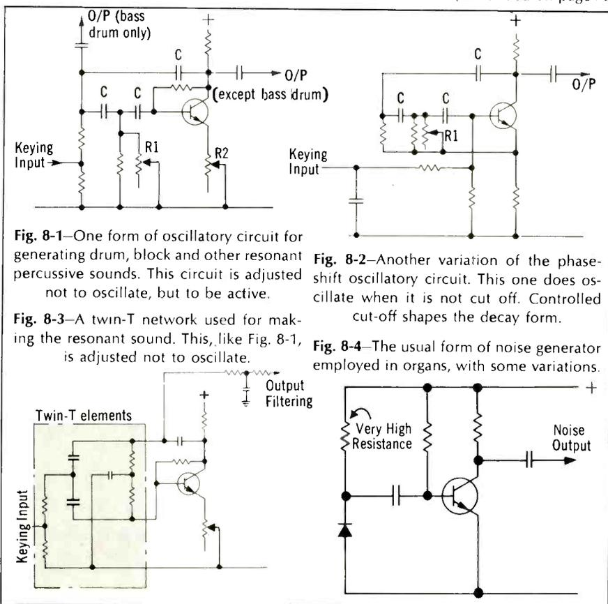
Fig. 8-1—One form of oscillatory circuit for generating drum, block and other resonant percussive sounds. This circuit is adjusted not to oscillate, but to be active.
