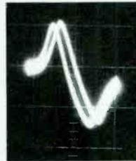
Fig. 11—Ratio-detector output not properly centered about "zero."
