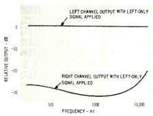
Fig. 6—Typical stereo separation curve
