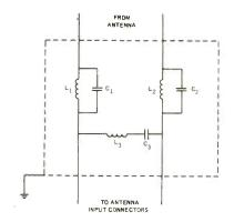
Circuits tuned to interfering signal. Fig. 2-Interference trap.
