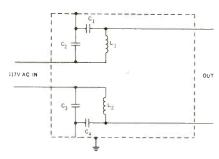
C<sub>1</sub>C<sub>2</sub>C<sub>3</sub>C<sub>4</sub> 500 pF mica.  $L_1L_2$  20 turns #18 enamelled wire on ½-inch dia. form, close spaced.
