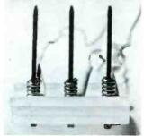
New solderless connection techniques: Tension-wrapped terminal connections plus plug-in circuit modules result in the kind of reliability associated with aerospace applications.
