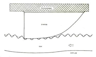
Fig. 3—Showing the shape of the stylus and the way it can glide over the grooves
