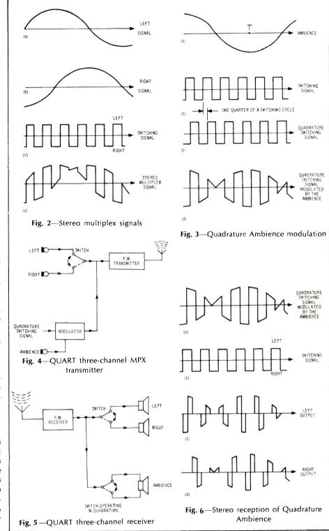
$$\frac{L+R}{2} + \alpha \sin 2\pi \text{ ft} + \left(\frac{L-R}{2} + \gamma\right) \sin 4\pi \text{ ft} + A \cos 4\pi \text{ ft}$$
