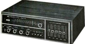
JVC Model 5010. Moderately priced AM/FM multiplex stereo. Has Advanced SEA with knobs that click up or down in 2db steps within a range of ± 12db, just like the more expensive models. 40 watts total dynamic power. Five IF stages. New FET reachs out for distant FM stations. 1% IM distortion. Accommodates 2 speaker systems simultaneously. Wood cabinet.
