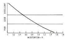
Fig. 9-Ratings for IM distortion
