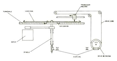
Fig. 2—The turntable drive system
