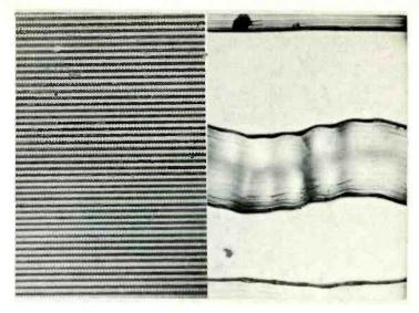
Fig. 1—Showing the groove pattern of a conventional record (right) compared with the dense grooves recorded by the FM system
