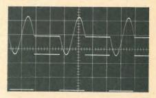
Fig. 3-Alternate single cycles of ON and OFF.
