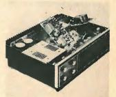
Hinged circuit boards for FM IF. AM IF. Multiplex and Phono Preamp sections - six plug-in boards for all other maior circuitry
