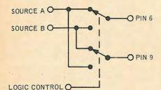
Fig. 7—The equivalent of the MC1496G as a DPDT switch.
