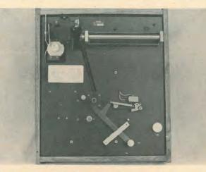
Fig. 2-Top view of the ST-4 with platter, arm, and mechanism cover removed to show the simplicity of the entire chassis.
