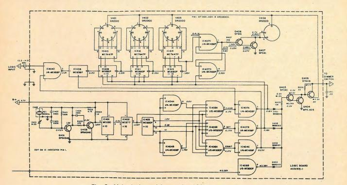
Fig. 2-Major logic module contains 100 kHz reference, or "clock" frequency crystal oscillator, further divides IC's and the necessary logic "gates" to drive the segments of the numeric read-out tubes.
