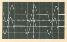
Fig. 4-The upper waveform advanced the lower retarded, with switching waveform not shown.
