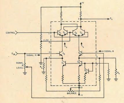
Fig. 6-The MC1496G connected up as a two-channel switch.
