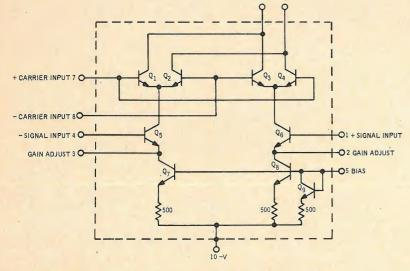
Fig. 5-Schematic of MC1496G balanced modulator/demodulator.
