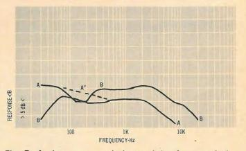
Fig. 7-A, Average spectral characteristic of concert halls, as actually measured without audience; A', predicted result with audience, and B, average spectral characteristic produced by AR-3a systems at 22 listening locations in eight living
