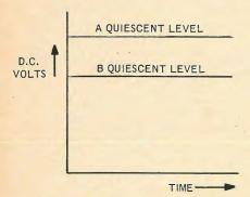
Fig. 8-Switching transients are due to the differences in the A and B quiescent levels.
