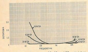
Fig. 6-THD versus frequency at 20, 40, and 50 watts/channel levels
