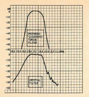
Fig. 3-Sherwood's published comparison between its i.f. bandpass response using multipole filters and "inferior" crystal filters. I.f. systems using conventional tuned interstage. transformers would probably suffer even more by comparison.
