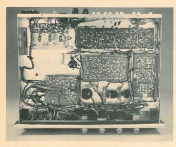
Fig. 5-Bottom view of the SEL 300 chassis
