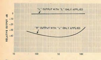
Fig. 7-Stereo FM separation characteristics.
