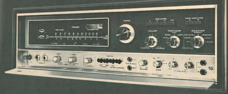
And if you want to get down to the nitty gritty, the SX-9000 has an FET front end with sensitivity at 1.6 microvolts to bring in the most fainthearted stations. There are 4 IC's in the IF; combined with a 1 dB capture ratio and 40dB selectivity, you can pinpoint stations on the most crowded
