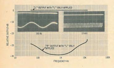
Fig. 3-Stereo FM separation.
