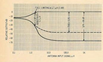
Fig. 2-Mono FM characteristics.
