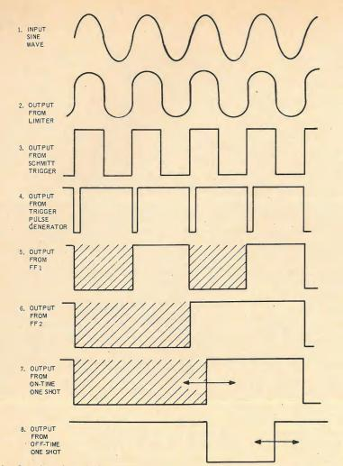
Fig. 10-Synchronizer timing waveforms.
