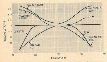
Fig. 7-Tone, filter, and loudness control characteristics
