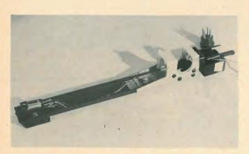
Fig. 1-Underside of arm, showing nylon guide rollers, counterweight, and the four-contact plug carrying the pickup output. Plug inserts in matching receptable on chassis, and four fine wires carry the signal from the cartridge with a minimum of drag on the arm.
