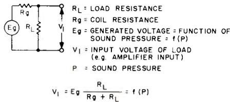
Fig. 1—Equivalent electrical circuit of a dynamic transducer.
