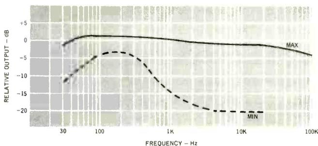
Fig. 5—Tone control and frequency response.
