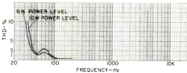
Fig. 3—Harmonic distortion at low frequencies.
