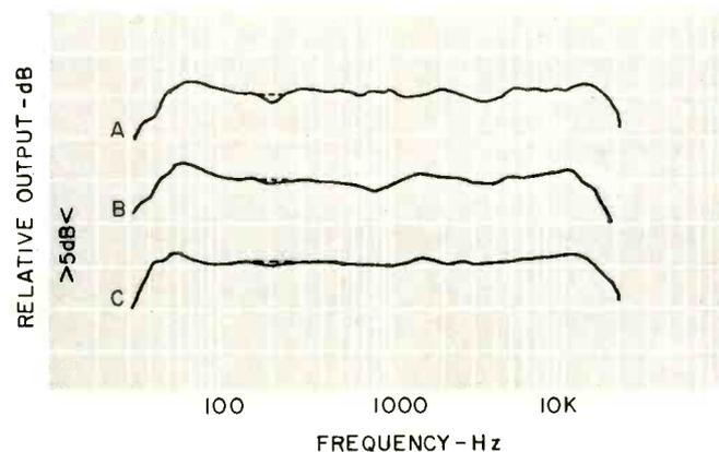
Fig. 1—Response curves with one-third octave pink noise; A is taken on-axis, B at 45 degrees off-axis, and C is an average of five angles.
