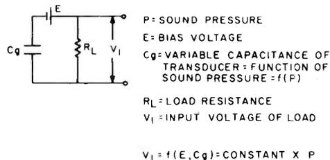
Fig. 2—Equivalent electrical circuit of a condenser transducer.
