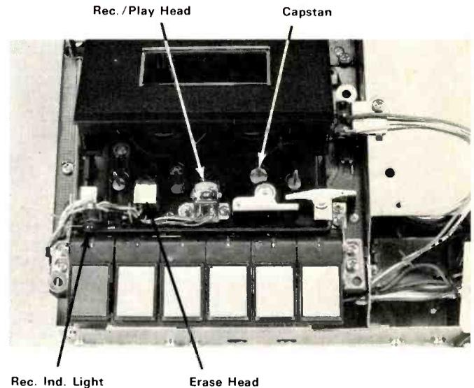
Fig. 1—View of the cassette compartment showing the positions of the two heads, the capstan, and the record indicator light.
