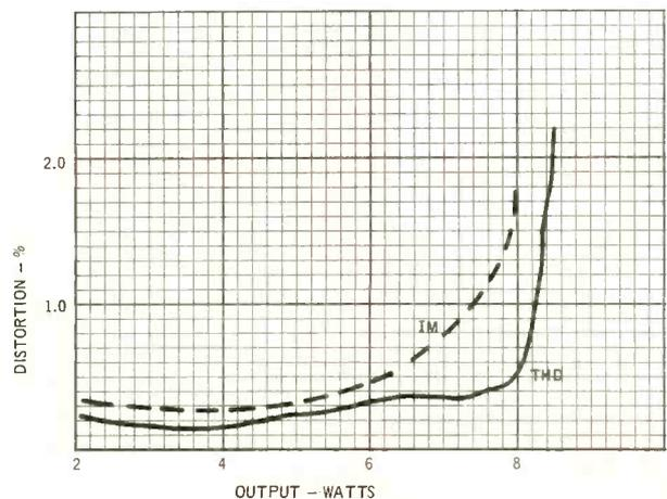
Fig. 4—Power Output, both channels driven (4 ohms).
