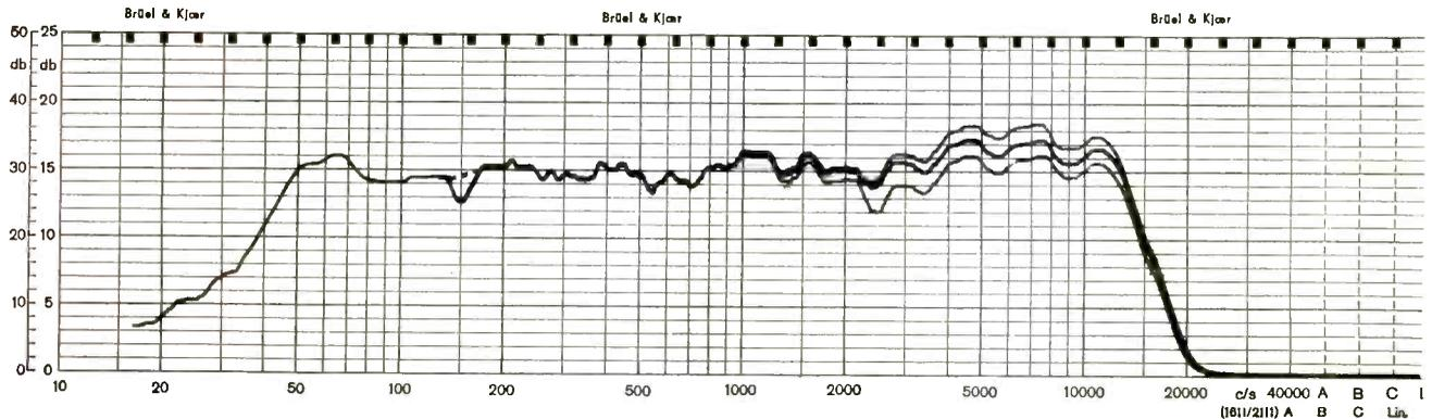
Fig. 2—Frequency response with the tweeter level control in three positions.
