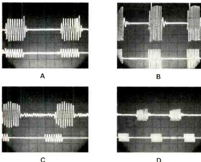
Fig. 4—Tone-burst response at A, 50; B, 100; C, 3000, and D, 10,000 Hz.
