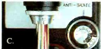
B. Made of modern, low-mass magnesium, the GT55's tonearm weighs an astonishing 14 grams. It rides on jewel vertical pivots and horizontal ballbearings. Inertial drag and friction are reduced to absolute minimum levels.
