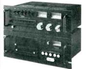
pitch control provides accurate tuning. The stated frequency response is 30 Hz to 18 kHz  $\pm$ 3 dB, wow & flutter 0.04 W rms, and weighted S/N ratio above 5 kHz w/Dolby of 65 dB. Price: \$1500.00.
