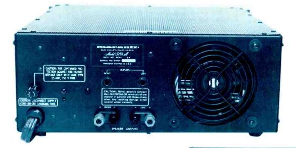
One fuse on the rear panel interrupts the a.c. line in case of amplifier failure, while external, in-line fuse holders are provided for speaker protection. In the owner's manual are diagrams showing the proper connections and guidelines for fuse selection. The use of these fuses is recommended.
