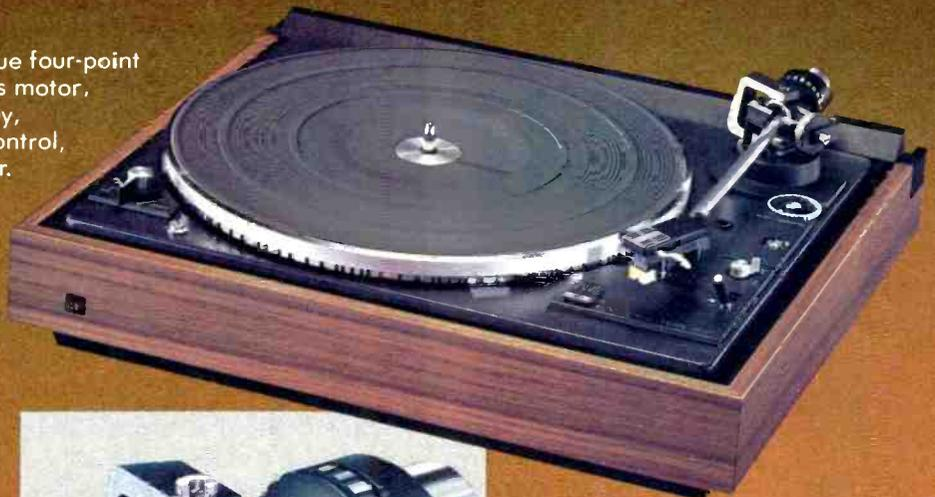
The four-point gimbal centers and pivots the tonearm mass at intersection of horizontal and vertical axes. Tonearm is dynamically balanced in all planes. The four needle-point pivots are first hardened, then honed, a process which produces microscopically smooth surfaces. The precision ball-bearing races are only 0.157 inch diameter. Bearing friction: vertical, <0.007 gram; horizontal, <0.015 gram.
