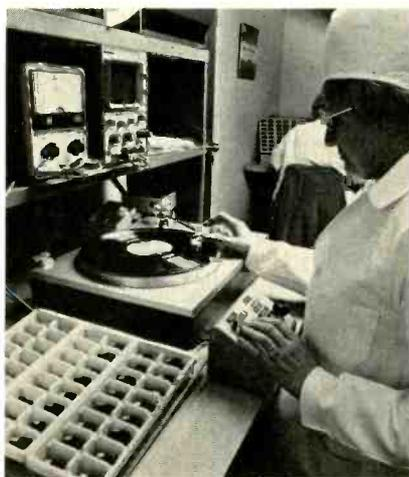
**11. 100% quality control of all cartridges.** All fully-assembled cartridges are individually played on a CBS STR-100 test record, monitored on a dual trace oscilloscope and measured with a VTVM.
