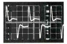
Fig. 4—Equalizer output with a 500-Hz square-wave input and the 2- and 4-kHz filters at +6 dB.
