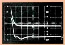
Fig. 5—Preamp output (top) with 1-kHz square-wave input and a +10-dB boost at 10 kHz with the tone control. Equalizer output (bottom) with the 1-kHz square-wave input and filters set to match the preamp frequency response.
