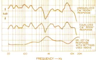
Fig. 3 - Equalization of room-like response.
