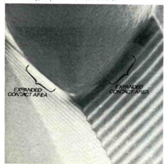
Scanning Electron Beam Microscope photo of Stereohedron® stylus, 2000 times magnification; brackets point out wider contact area. © Stanton Magnetics, Inc., 1977
