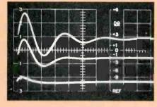
Fig. 1—Equalizer output with a 500-Hz square-wave inut, with the 3600 filter at +4 (bottom), + 8 (middle), and +12 dB (top).
