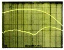
corresponds to 3.42 watts. The 10 per cent total harmonic distortion point occurred with a power output of 4.62 watts, lower than the 6 watts per channel claimed by the manufacturer
