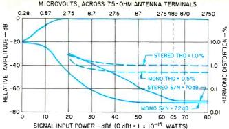
Fig. 1-Mono and stereo quieting and distortion characteristics for the FM section of the Sanyo FT-1490A.
