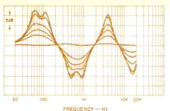
Fig. 2—"Flat" response and the settings of 3, 6, 9, 12, & 15 dB for 63 and 125 Hz (+), 500 and 1000 Hz (-), 4 kHz (+), and 16 kHz (-).
