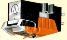
Magnet construction provides a *separate* magnetic system for *each* stereo channel. A concept that insures excellent stereo separation, while lowering magnet mass. And the AT12XE features a tiny 0.3 x 0.7-mil nude-mounted elliptical diamond stylus on a thin-wall cantilever to further reduce moving mass where it counts. Each cartridge is individually assembled and tested to meet or exceed our rigid perform-
