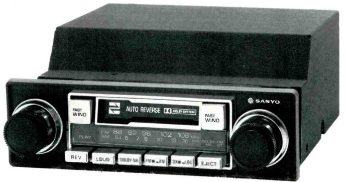
The first thing we learned about the Sanyo FT-1490A is that it is equipped with separate amplifier sections for woofers and tweeters and therefore qualifies as a "bi-amp" unit. It is also one of the few car units we have seen which is equipped with Dolby noise reduction circuitry in its cassette section. Aside from that, we were left largely on our own as far as
