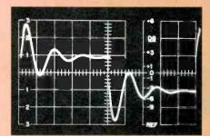
Fig. 3—Equalizer output with 270-Hz square-wave input with the 1800-Hz filter at +12 dB.
