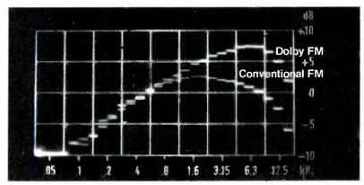
Real-time analysis of the output of a Dolby FM receiver tuned to interstation noise. This is equivalent to a station broadcasting "white noise," a test signal containing a great deal of high frequency energy, which is represented graphically by a rising straight line. The curves show that Dolby FM can provide much more high frequency information at high levels.
