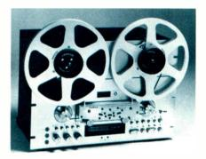
ulated tension between the capstans. Logic circuitry prevents more than one control button being pushed at a time. The unit features a 4-track, 2-channel design, and the user can record on one or both of the channels. At 7½ ips, its specified S/N is more than 60 dB, harmonic distortion less than 1 percent, frequency response 20 Hz to 20 kHz, and wow and flutter 0.04 percent. Price: \$895.00.
