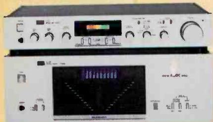
**B-77 LINEAR-A DC Servo Power Amplifier with Spectrum Analyzer and Peak Power Meter.** Sensibly rated at 60 watts/channel, min. RMS, both channels into 8 ohms from 20-20,000Hz, with no more than 0.03% THD. Direct-coupled throughout, it features Sansui's exclusive new "Linear A" circuitry for low distortion with high efficiency, along with separate 10-band spectrum analyzer and peak power displays that show just what your system is doing.
