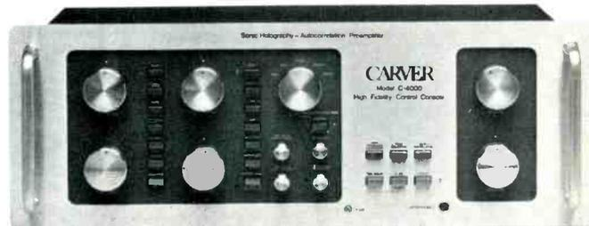
**The C-4000** Control Console includes the Sonic Hologram Generator plus: a full-function stereo preamplifier, a time-delay system with built-in 40 watt (total) power amplifier for time delay speakers, the Autocorrelator system that reduces noise up to 8 dB with any source material, and a peak limiter/downward expander that nearly doubles dynamic range.
