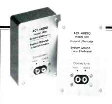
The Ace Audio Model 3900, which is designed to eliminate ground loops in high-fidelity systems, is actually a very simple device. It is a small box with two phono jacks, input and output. The center, or signal, terminals are bent and soldered together, and the input shield/ground is tied to the metal mounting plate. The output ground, however, is not connected to the input ground or the box plate in any way. In this fashion, the
