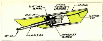
Fig. 1 — Cut-away view of the V-15 Type IV cartridge, courtesy Shure Bros.
