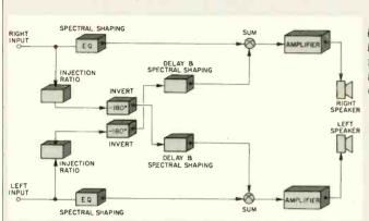
Fig. B2—Basic block diagram of the Sonic Hologram Generator.
