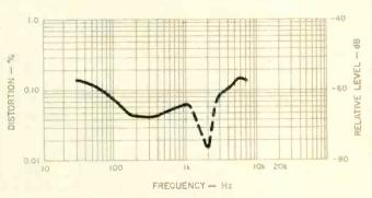
Fig. 6—Third harmonic distortion vs. frequency in Dolby mode at 10 dB
