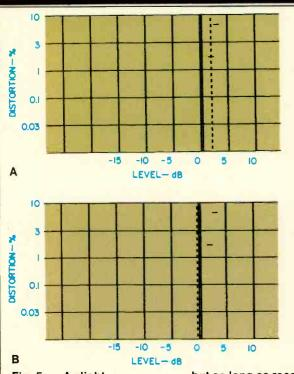
Fig. 5 — A slight improvement in 3rd-order harmonic distortion was noted when 16-bit mode is used on Sony PCM-F1 (A),
