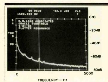
Fig. 10—Spectrum of platter resonance. See text.
