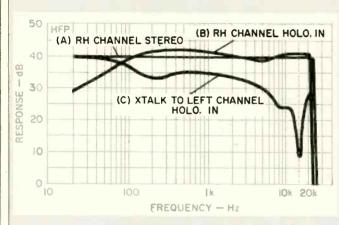
Fig. B3---Frequency shaping in the Hologram Generator: (A) Response in standard stereo. (B) contouring on main channel through Generator, and (C) relative level and contouring on crossfed signal. Chart recorder causes roll-off above 20 kHz.
