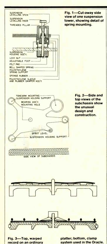
which allows dish-warped records to be flattened and fastened securely. The mat is made of a special composition designed to absorb mechanical vibrations from the record. These vibrations, a result of the stylus interaction with the record groove, have been largely ignored until recently. Such vibrations travel back and forth within the record, forming delayed reflections of mechanical energy, which, if not damped quickly, are picked up by the stylus and blur the detail of reproduced sound
