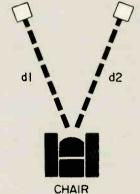
Fig. B1—Setup for sonic holography. Make d1 and d2 as close to equal as possible.
