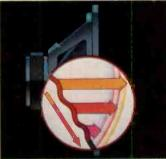
Ohm Walsh 2™ loudspeaker -- single arrow represents pulse travelling down inverted surface causing in-sync fragments (as represented by 3 horizontal arrows) to enter air along the way eliminating the problem of stereo ghosts. Enter No. 16 on Reader Service Card
