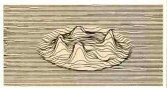
Fig. 6B—A highresolution plot at 14,274 Hz shows a severe, fourpole bell mode.
