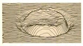
Fig. 5B—At 1022 Hz, laser-computer animation reveals a rocking mode,
