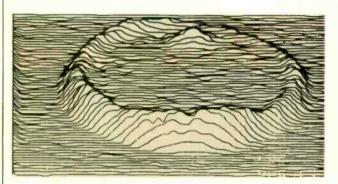
Fig. 2B—Ultra hard metal dome shows asymmetric decoupling of its surround at 8kHz.
