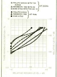
Fig. 7—HDL<sub>3</sub> vs. recording level at 200 Hz and 4 kHz for three recorder-tape combinations.
