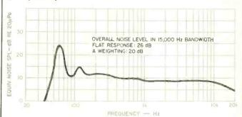
Fig. 7—Microphone noise spectrum (one-third octave bands) of AT813.
