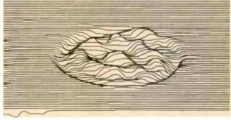
Fig. 6C—At 21,031 Hz, the bell mode is eighth-order, but with less effect than the 14,274-Hz mode.
