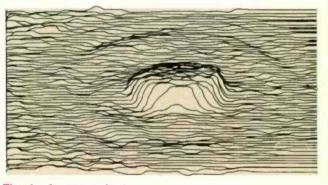
Fig. 4—A severe dustdome problem shows up in the bass/mld unit at 1.3 kHz.
