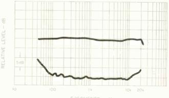
Fig. 2—Frequency response and separation.
