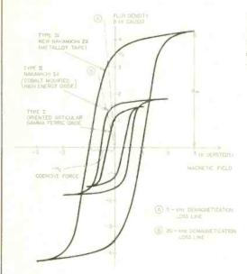
Fig. 1—Hysteresis loop characteristics of three cassette tape formulations.
