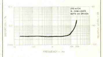
Fig. 2—THD vs. frequency at rated output.
