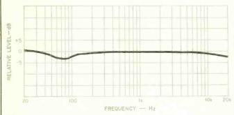
Fig. 2—Frequency response loss due to loading of our microphone preamp.
