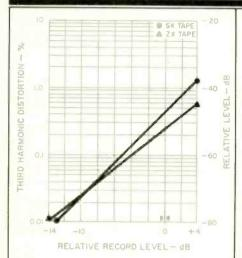
Fig. 6—HDL<sub>3</sub> as a function of recording level at 1 kHz with Nakamichi SX and ZX tapes on 700ZXL recorder.
