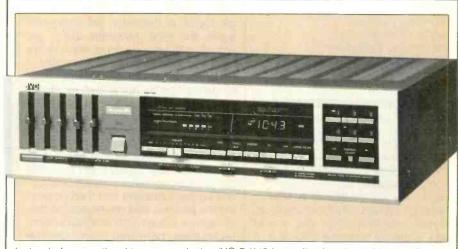
Instead of conventional tone controls the JVC R-X40 has a five-band graphic equalizer
