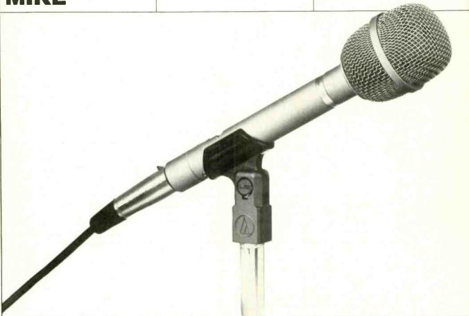
The Audio-Technica Model AT813 is a cardioid unidirectional electret microphone powered by an internal battery. It was designed for audiophile or professional recording applications, or sound reinforcement. The large metal screen on the head end encloses an integral wind/pop screen. The
