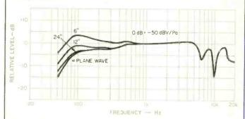
Fig. 5—Frequency response vs. distance from source (sample #1).
