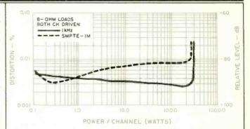
Fig. 1—Distortion vs power output, Heath AA-1800 power amplifier.
