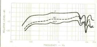
Fig. 6—Frequency response vs. angle (sample #1).
