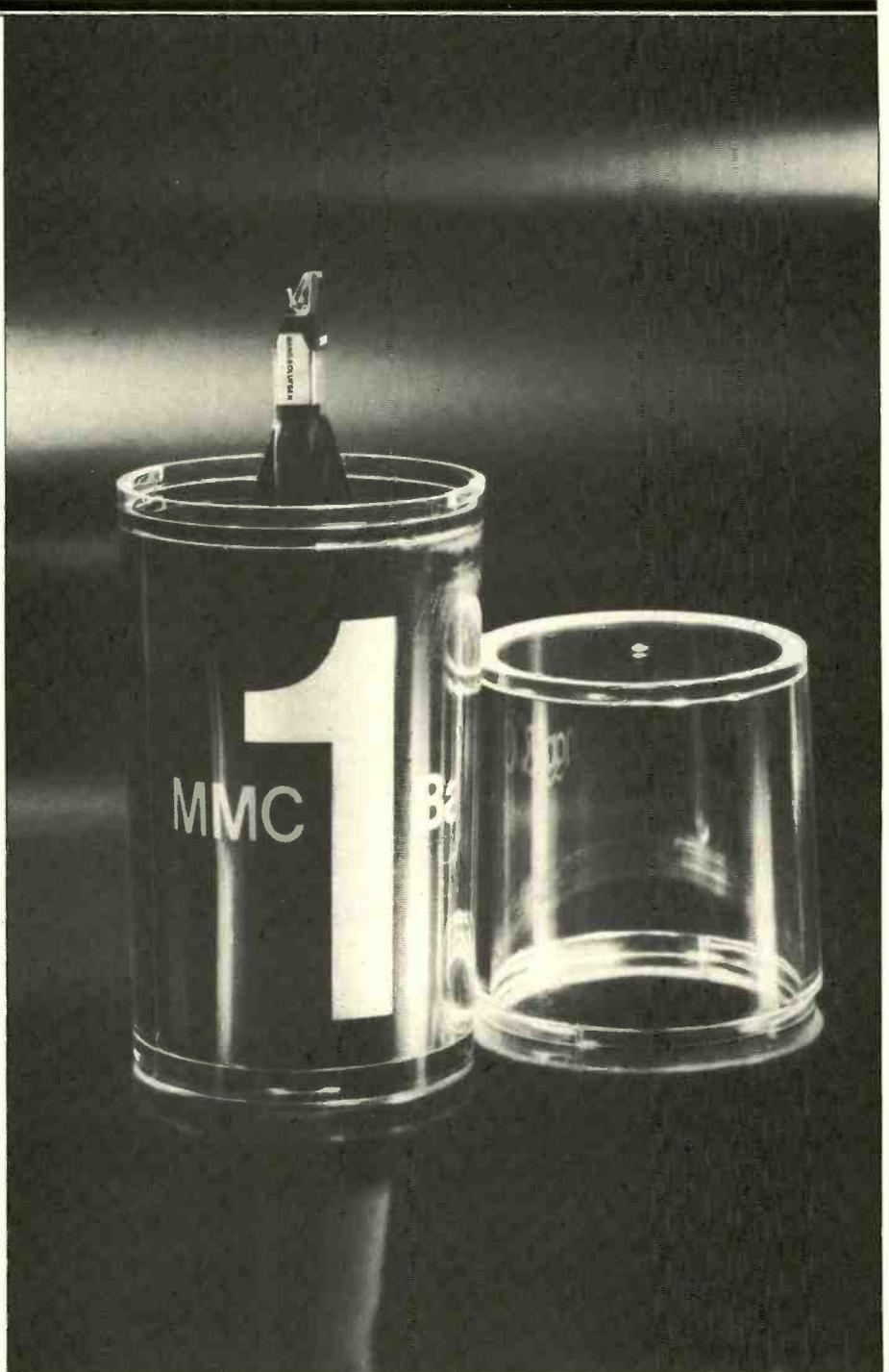
Bang & Olufsen (B & O) has recently introduced a new series of five phono cartridges, and the MMC 1 is the top of the line. They also seem to have refined their well-established moving-iron generating principle, called the "moving micro-cross" (MMC), which transforms mechanical energy to electrical energy. The X-shaped moving micro-cross armature moves within the magnetic field created by the
