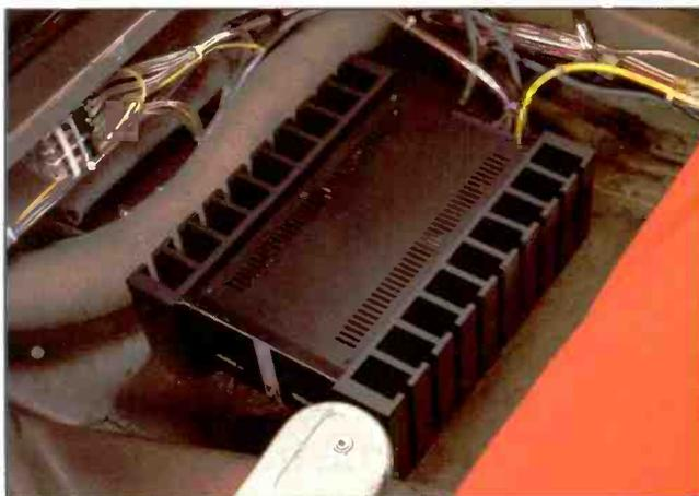
This Alpine 3502 amp, beneath the back seat, can be switched from the dash to handle ADS 320i speakers in the doors or rear-deck speakers under test. It's the only amplifier powered with ignition in "Accessory" position—the amp rack is only on when the motor's running.
