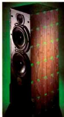
The technique of modal analysis enables enclosure wall vibration to be examined by taking measurements at a number of points.
