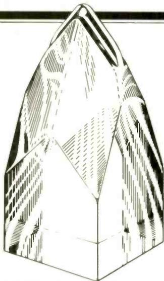
The tall, thin "footprint" of the Signet's MicroLine stylus scans fine details well.
