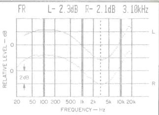
Fig. 2-Same as Fig. 1 but treble dips are -2.1 to with Time Lens on. Bass peaks shown measure +2.3 to +2.4 dB at 145 Hz.
