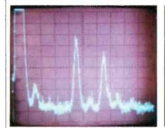
Fig. B8—Spectrum analysis of waveform shown in Fig. B6 shows high level of harmonic distortion components.
