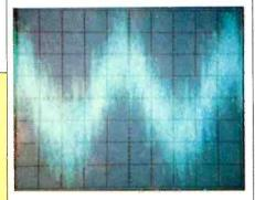
Fig. B7—Same as Fig. B6, with dither added before D/A conversion.
