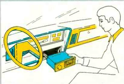
*Fig. C1—To check on whether noise is being induced into the receiver, pull it from its mountings while it remains connected, and listen for a drop in noise level.*
