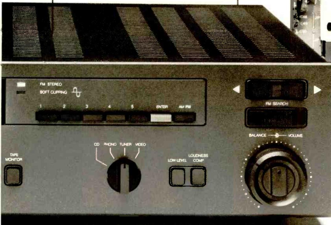
**CD Input.** The 7130 receiver has a separate CD input (not merely a re-named AUX input) for a Digital Compact Disc player. There is no input circuit that could be overloaded by high level peaks; the signal goes directly to the Volume control before it is amplified.
