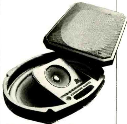
*Most car speakers are flush-mounted in holes cut into the car's interior panels. Since oval speakers are usually mounted in the shelf behind the back seat, some models (such as the Coustic HS-892, shown here) tilt the tweeter up to aim it more directly at the listener.*
