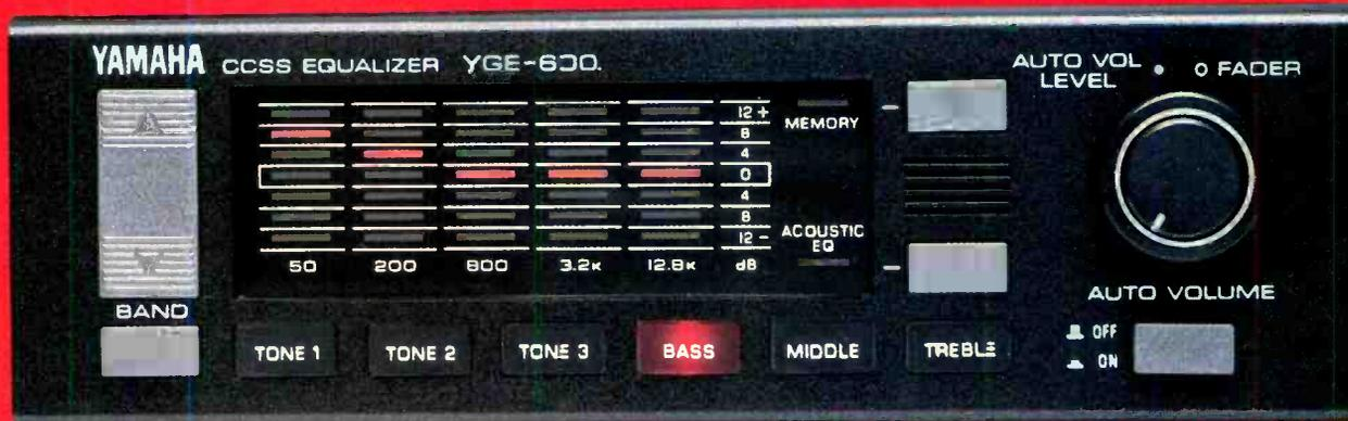
The Auto Volume circuit worked smoothly, especially once I had adjusted its front-panel setting. In my car, which is fairly noisy, the system worked best with the control nearly at its maximum. The automatic adjustment range is deliberately limited: Yamaha's instruction manual shows a level change of only 14 dB for a 20-dB change in ambient noise.
