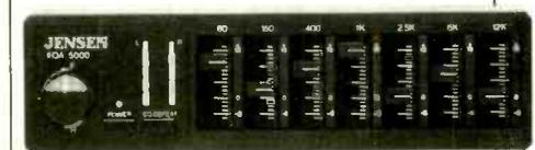
*Equalizers with up to seven bands are still simple enough to be used as extra-versatile tone controls.*
