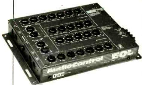
*Complex equalizers should be set up by a competent installer, preferably with the aid of test instruments, and then left alone. Such equalizers are often mounted in the trunk to discourage fiddling.*
