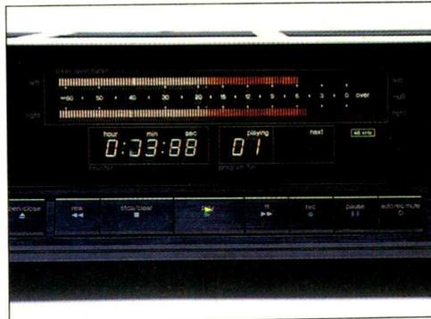
The yellow and red segments on the Technics SV-D1000's recording meter help warn the user when levels approach the point of overload distortion.
