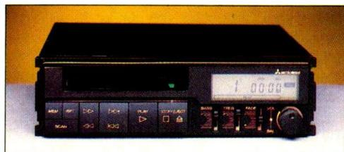
vances from one recorded selection to another, stopping and playing the first 10 S of each before advancing to the next. Pressing the "Play" button at any time disengages "Scan" and allows you to listen uninterrupted to the selection of your choice. Considering that a DAT cassette may contain as much as two hours of recorded material, this is a very useful feature, allowing a driver to audition many selections without having to repeatedly take his hands off the wheel.
