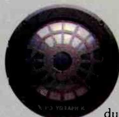
For the frequency range of 85 Hz to 700 Hz we developed a unique transducer which we call Polygraph™. This 5" dome-shaped driver is made of very thin polypropylene supported by an extremely light, stiff lattice of graphite. Its transient response in the midbass and lower midrange — the area of most musical fundamentals — rivals that of the most expensive planar drivers. Its power handling and dynamic range surpass them.
