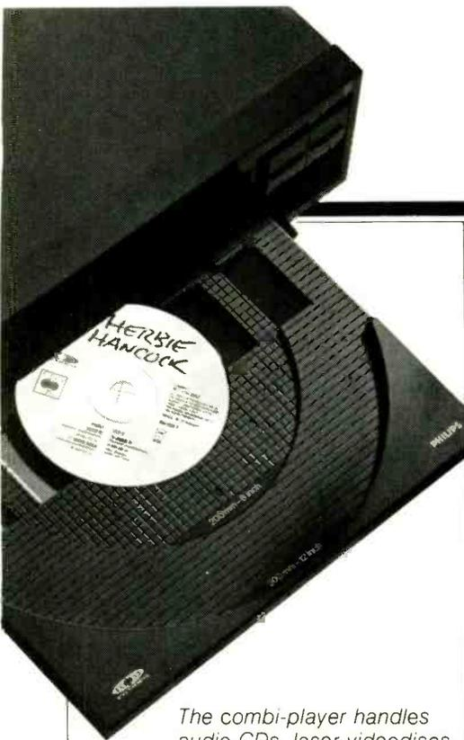
The combi-player handles audio CDs, laser videodiscs, and new CDV-Single discs.
