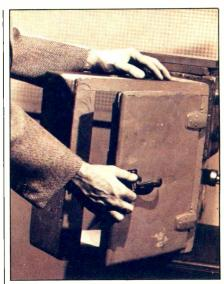
Following scripts closely, the soundeffects men would slam doors, which sometimes were the real thing simply brought into the studio and mounted. In other cases, miniatures were built specially for the purpose.
