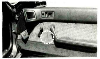
Passenger-side door with 751 system: (left) angle-mounted 1" Varimount tweeter; (circled) 51/4" woofer mounted behind fabric.
