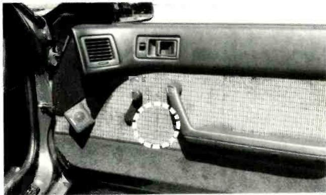
Passenger-side door with 751 system: (left) angle-mounted 1" Varimount tweeter; (circled) 5/4" woofer mounted behind fabric.
