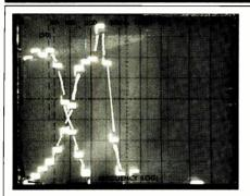
Fig. 6—One-third octave spectra of warble tones at 31.5 and 250 Hz. (Vertical scale: 5 dB/div.)
