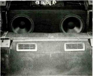
Before-and-after view of custom-made enclosure for 780LF 8" subwoofers.
