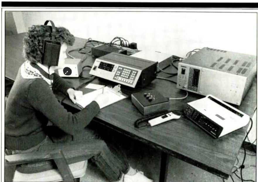
*In the National Bureau of Standards' parallel listening tests, subjects were asked to pick out which of two recordings had been encoded with the Copy-Code notch, by reference to a third, unencoded recording. The average percentage of correct identifications was 62.3%.*
