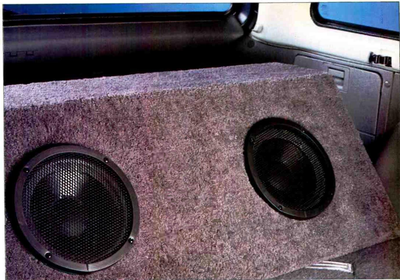
Two views of the subwoofer enclosure show that it does not intrude terribly into the cargo space, despite having a fairly large volume. Note the amplifier fins emerging from the enclosure as well as the quick-disconnect plugs. (The shiny diagonal on the floor is a cargo tiedown.) The front tweeters were flush-mounted in the doors, while tweeters for the rear system were hung from the roof, pointing forward toward the passengers.
