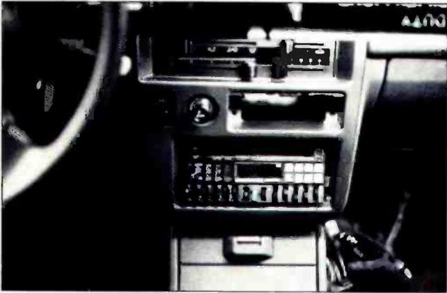
**The dashboard radio slot was gradually enlarged to be a snug fit for the new Alpine electronics.**
