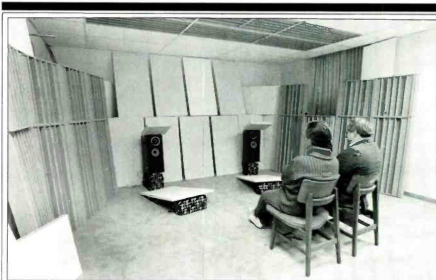
*The NBS listening room used sound-absorbing materials on the wall behind the speakers, on the side walls, and on the ceiling; sound-diffusing panels were used on the fourth wall (not shown). Only two subjects were allowed to listen at a time.*
