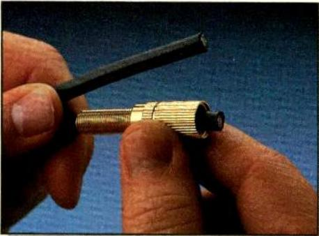
**Step 2** – Insert the cable through the rear half of the connector until it extends about 1/8 inch.
