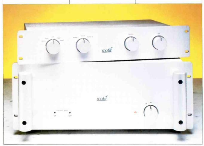
The MS100 and MC8 are among the top pieces of audio electronics manufactured by Motif, of conrad-johnson design. The MC8 preamplifier is an all-FET design which is unusual in at least one sense: It does not use any electrolytic capacitors in its circuitry-even in the power supply. The MS100 power amplifier is rated at 100 watts per channel into 8-ohm loads and uses a combination of junction and
