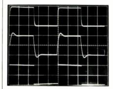
Fig. 11—Amplifier response to square wave. Top trace is 10 kHz with 8-ohm resistive load. Middle trace is 10 kHz with 2-μF capacitance across 8-ohm load.
