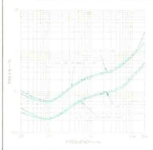
Fig. 1—THD + N for MM phono section of MC8 preamp, measured at tape out.
