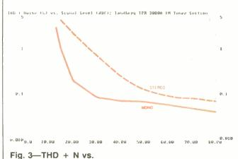
signal strength for a 1-kHz modulating signal.
