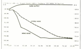
Fig. 2—Mono and stereo quieting characteristics.
