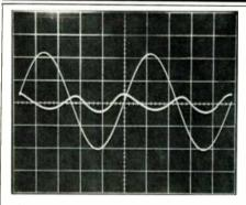
Fig. 9—Response to 10-watt, 1-kHz sine wave. Distortion products
