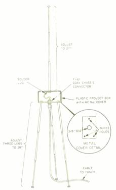
Fig. 1—Construction diagram.
