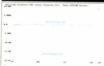
Fig. 2—Frequency response of main stereo channels with a mono input. The high-frequency
