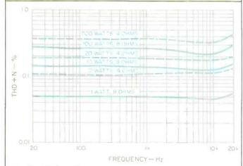
Fig. 7—THD + N vs. frequency for MS100 amp, at various power levels, into 4 and 8 ohms.
