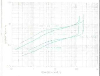
Fig. 8—SMPTE IM and THD + N vs. power for 4 and 8 ohms. THD + N is for a 1-kHz test signal,
