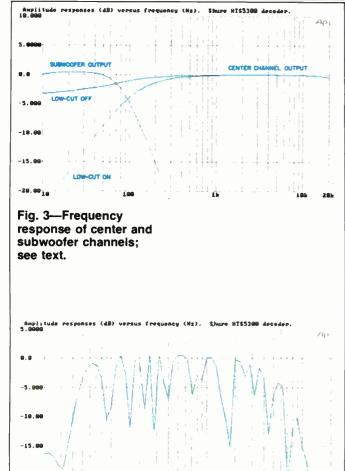
Fig. 4—Frequency response of surround channel, with left and right inputs of opposite polarity. The comb-filter effects shown are normal
