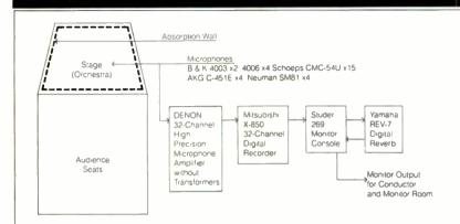
Fig. 2—Setup for Denon's anechoic recording.
