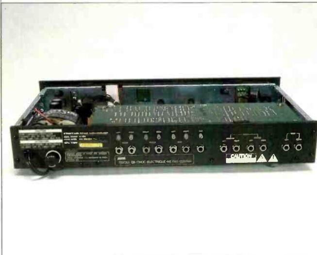
The Proton processor senses how many channels are plugged into it, then automatically adjusts its action to match.
