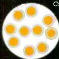
Cross section of Museatex speaker cable showing individually insulated, 24 gauge, oxygen-free copper wire in loosely twisted pairs. Note that the copper wires do not touch each other.
