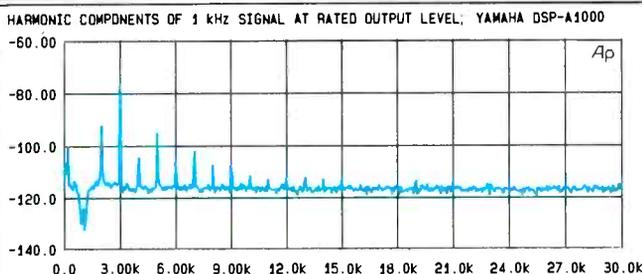
**Fig. 5—Spectrum analysis of harmonics of 1-kHz main-channel signal at 80 watts per channel into 8 ohms. Curve shown is averaged result of 16 acquisitions, to reduce displayed noise and improve display of coherent signals.**
