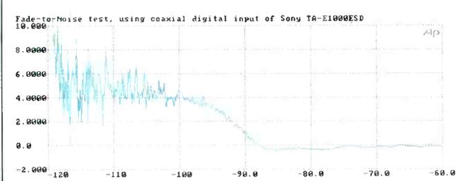
**Fig. 7—Fade-to-noise test of D/A converter section.**
