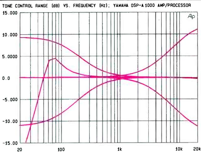
Fig. 7—Bass and treble control range, plus action of "Bass Extension" circuit.
