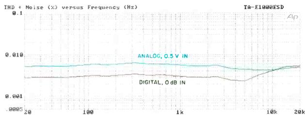
**Fig. 3—THD + N vs. frequency for analog and digital input signals.**
