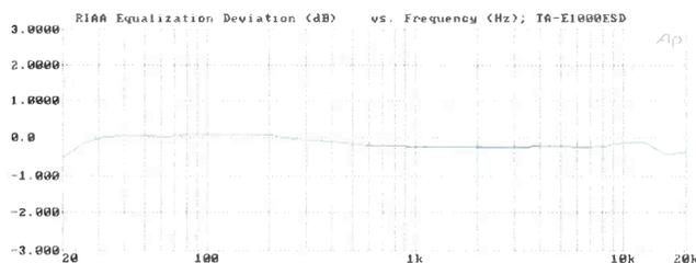
**Fig. 2—Deviation from RIAA equalization.**
