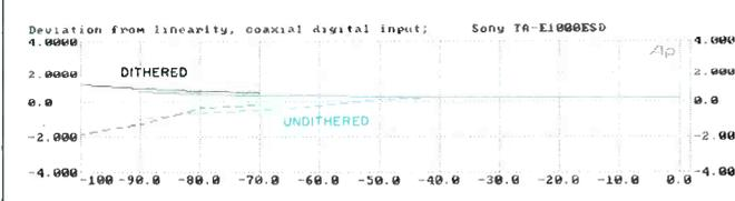
**Fig. 6—D/A converter deviation from linearity, for dithered and undithered signals.**
