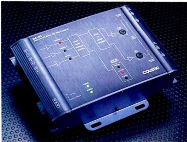
The DA-55 utilizes a U.S. made Dual Single-Bit Chip Set design with 18-Bit Resolution, which incorporates a Dual 8 Times Oversampling Digital Filter, a 64 Times Oversampling Fifth Order Delta-Sigma Modulator, as well as an Ultralinear Digital to Analog Filter Set (a Fourth Order Butterworth Switched-Capacitor Filter with multiple feedback loops followed by a Second Order Butterworth Analog Filter). The Filter
