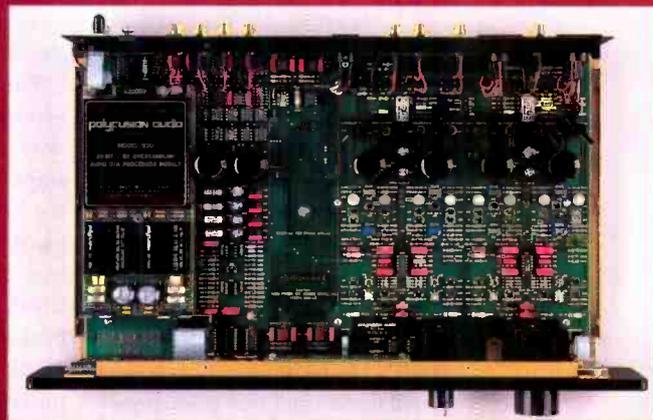
**DIGITAL INPUTS** Yes the 940 can be configured with Direct Digital inputs, with the optional 20-bit, 8 times oversampling DAC module, providing both coax and optic inputs. This is the same converter module which is the heart of our highly acclaimed models 800 and 900 off board DACs.
