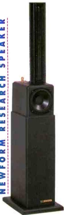
Towering atop the Standing Module 15 from Newform Research is a monopole ribbon tweeter, 15 inches tall and 3/4 inch wide, designed to offer transparent, open sound and a well-focused soundstage. Below it is a 5-inch woofer in an enclosure with a compact 6 x 9-inch footprint. Response is rated as 68 Hz to 20 kHz, ±2.5 dB, so the manufacturer suggests the system be used with a subwoofer. Price: \$945 per pair; delivered direct from factory. For literature, circle No. 100
