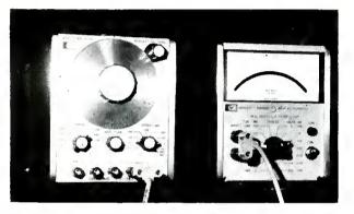
**Hewlett-Packard.** Model 204D is the latest low-distortion audio oscillator and model 400F designates a high-sensitivity a.e. vtvm. Circle 34 on Reader Service Card.
