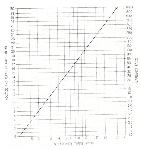
Figure 2. Transformer nomograph.
