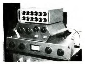
**Parasound Orban Associates.** In the middle, a new stereo synthesizer, below a compressor, above a control mixer. Circle 37 on Reader Service Card.
