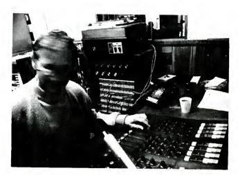
Figure 1. The author seated at the audio console of one of Hollywood Video Center's studios. Cartridge and reel-to reel recorders are just out of sight behind him. The glass looks into the studio proper but offers a poor view of the stage. A video monitor above the console shows the picture that is up.
