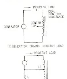
(B) GENERATOR DRIVING RESISTIVE LOAD
