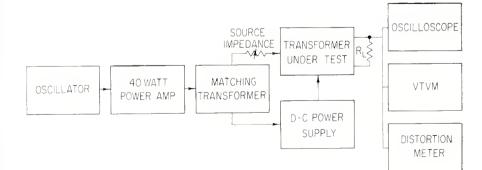
Figure 5. The transformer test set-up used at United Transformer Company.
