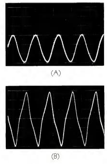
Figure 4. (A) The output waveform below maximum power capability is shown above; (B) the output waveform when the core is in saturation is below.
