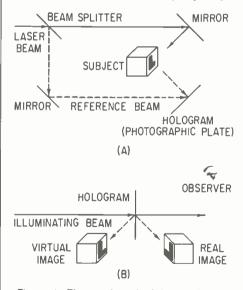
Figure 1. The usual method for producing and illuminating a 3D hologram.
