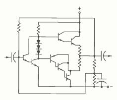
Figure 4. Most of the components shown appear on an integrated-circuit chip. This is a 1-watt power amplifier.
