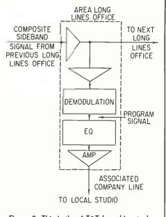
Figure 3. This is the AT&T branching technique.
