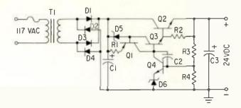
Figure 3. A power supply for the preamps described. The components are listed in Table 1.
