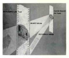
Figure 5. Production of a holograph from film, depicted in simplified form.
