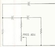
Figure 6. Making frequency adjustable is best achieved by putting a variable resistor in the middle phase-shift stage. Using a combination of fixed and variable resistance limits variation of oscillation condition within a practical range.
