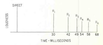
Figure 5. The time distribution of direct and first-order reflections.
