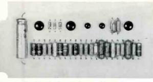
Figure 6. The Model 104 phono preamplifier card.
