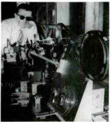
Figure 4. RCA scientist Robert A. Bartolini looks at equipment developed for making master holographic tapes for RCA's Selecta-Vision process.
