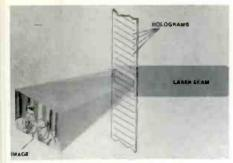
Figure 7. A simplified reconstruction of an image from the hologram tape.
