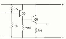
Figure 3. The Darlington circuit.  $R_{15}$  and  $R_{16}$  adjust the bias of the entire circuit.  $R_{17}^*$  can be used for more stable biasing.
