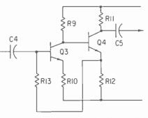
Figure 2. The invention of directly-coupled stages greatly simplified the circuit of Figure 1.
