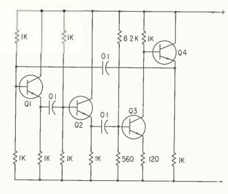
Figure 2. One way of embodying (as the patent specs say) the phase shifts of Figure 1 into a transistorized oscillator.
