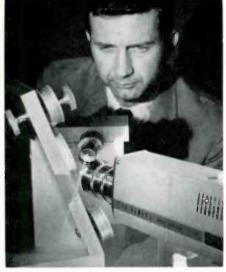
Figure 8. The basic elements of RCA's SelectaVision are demonstrated with lab elements by Charles Carroll. Directly in front of him is a low-power gas laser, sending a beam at the tape of a simple tape-transport mechanism (left). As the laser passes through the tape holograms, it bends part of it into the camera where it is deciphered into the final images.
