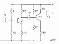
Figure 1. A typical class-A amplifier with two independent stages such as were first used with transistors.
