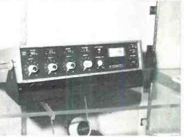
Shure Brothers offer this portable gated compressor for recording and broadcast use. Circle 73 on Reader Service Card.
