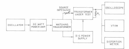
Figure 5. The transformer test setup as used at United Transformer Company.
