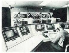
Figure 1. This is the origination studio of Trans-World Communications. Each of the seven cities in which the company operates has an identical control point which transmits current motion pictures to all the hotels hooked to the system. The "mini-computor" in the foreground transmits the selected features to the guest's room within 33 milliseconds of receiving the order.
