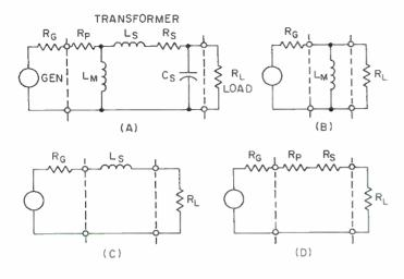
Figure 3. At (A) a simplified equivalent transformer circuit is shown, (B) is a low-frequency equivalent circuit, (C) a high-frequency equivalent circuit, and (D) is an efficiency equivalent circuit.
