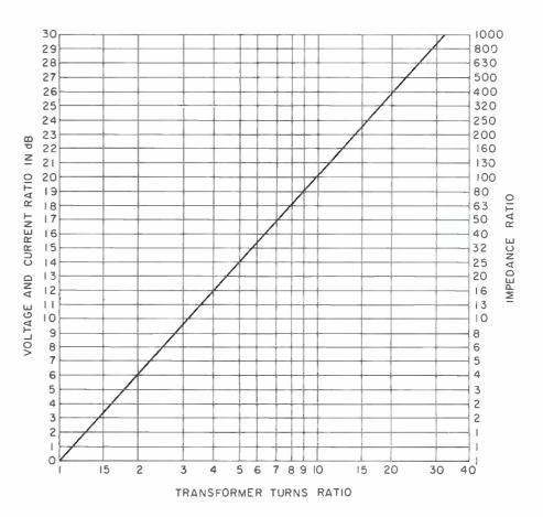
Figure 2. A transformer nomograph.
